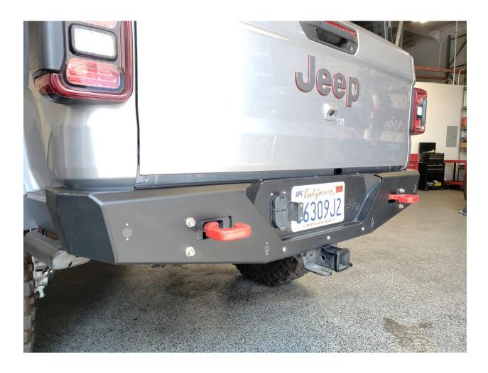
Be cautious of sensor wiring. Do not pinch wires when installing bumper. Connect Wiring to sensors and hitch plug, lights
