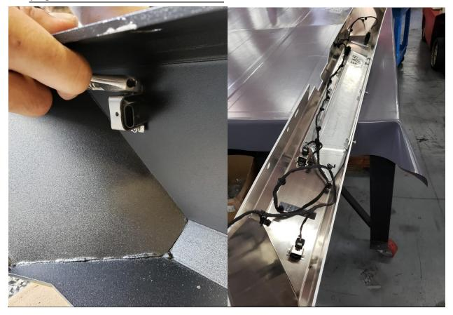
Careful when installing sensor hardware. Use a well fitted wrench and lightly tighten.
