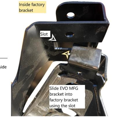
Insert EVO MFG Trackbar bracket into factory bracket, Use picture as reference.
