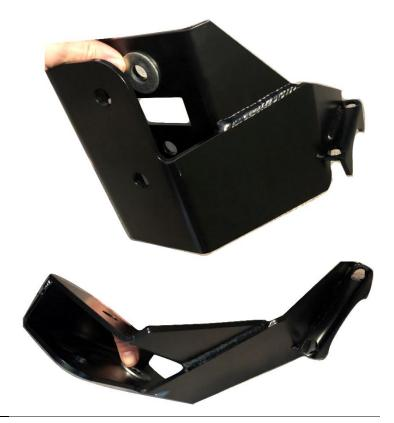
Line up bolt holes on EVO MFG bracket with the factory bolt holes. Loosely install provided hardware through the brackets.
