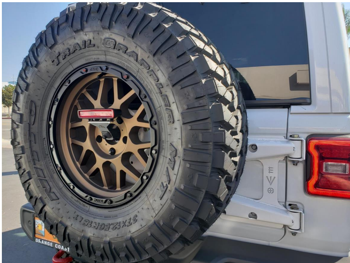
43. Install Camera with brakelight bracket on top using factory screws to camera tube.
