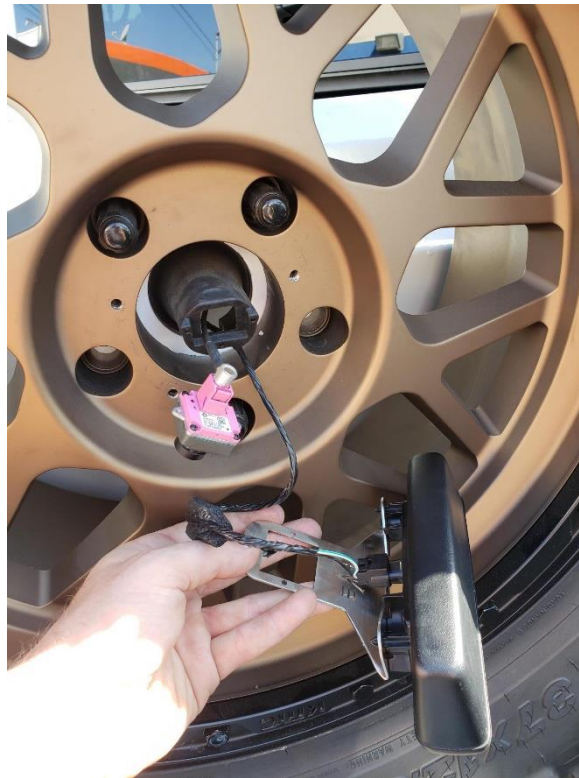
43. Install Camera with brakelight bracket on top using factory screws to camera tube.
