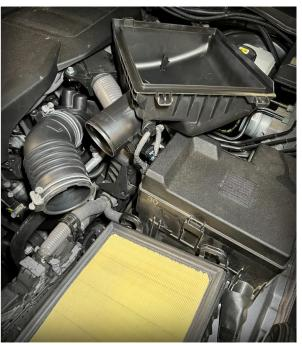
Pull the air box housing up and out of the vehicle to expose the ECU mounting bracket.
