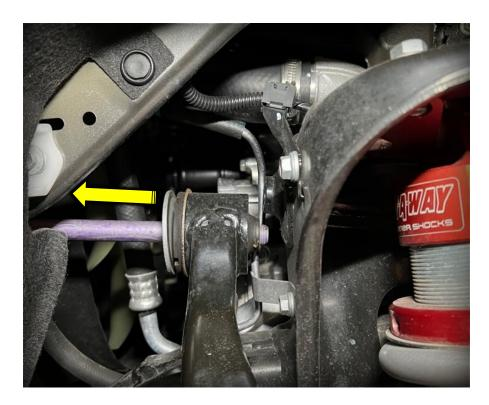
All that is left is to spin the ball joint castle nut off and remove the factory arm from the vehicle.
