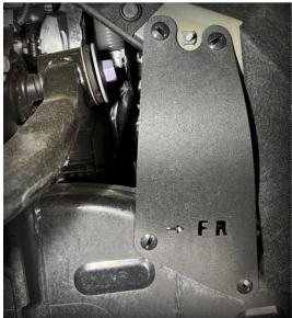
There is only one wire harness mount that needs to be unbolted to allow the cross bolt to come out towards the front. Repeat step 8 for this side and the arm will be out.
