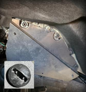
In order to get the cross bolt out on the **LEFT** (**DRIVER**) side, you must remove the intake airbox and ECU.
