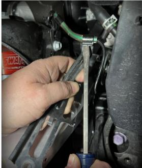
3 Unbolt the brake line brackets from the steering knuckle and frame.
