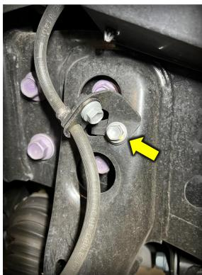
Remove the factory cotter pin using a pick. Loosen but do not remove the castle nut. Leave about a 1/4" of gap between the upright mount and nut.
