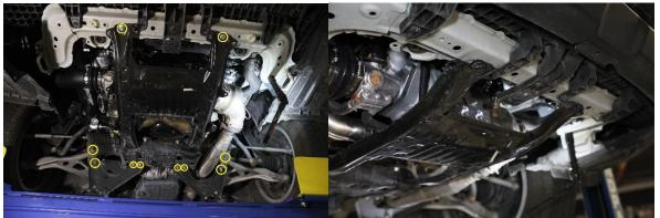
6. Install the Passenger Side Bumper using the (2) M8 Bolt, (2) M8 Flat Washer, (2) M8 Lock Washer, (1)1-1/8" Washer, and (2) O.E. Bolts. Sandwich the Under Guard between the Frame and the Bumper When Tightening Down the Hardware.
