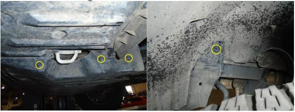
3. Remove the (8) pop clips & (2) Bolts located on the underside of the Under Cover Front.
