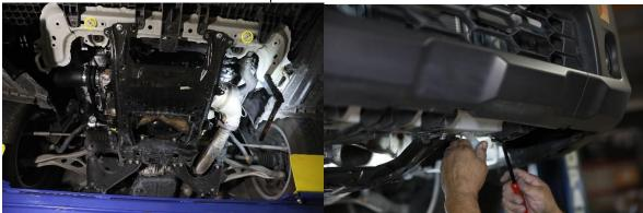
5. On the underside of the vehicle remove the (10) Bolts. Remove the Under Guard Front from the vehicle.
