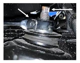
6. Using a **17mm** socket loosen and remove the stock lower shock mounting bolts. Save the stock lower shock mount bolts, as you will be re-using them with your new Sway-A-Way shocks.
