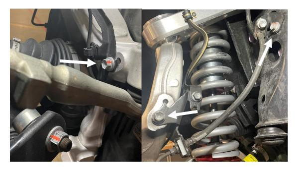
9. Remove the four (4) upper strut mount nuts (14mm).
