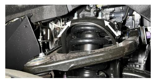
10. Remove the retaining clip, then loosen, but don't remove, the upper ball joint nut (19mm).
