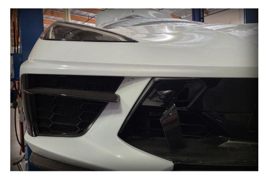
2 Install the tow hook stem into the factory threaded hole. The male threads of the stem are pre-coated with Vibra-tite. Both the stem and bolt threads are pre-coated with Vibra-tite threadlocker. This keeps your tow hook from loosening due to vibration. The special threadlocker is designed to remain flexible, removable, and reusable. Fully tighten stem with a 7/8" or 22mm socket.
