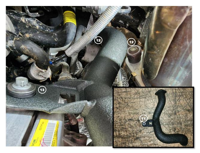
14. Transfer the mounting grommet from the factory upper hot side charge pipe to the supplied aFe upper hot side charge pipe in the same orientation as removed (11)
