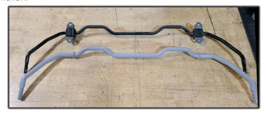
Lube the inside surface of the bushing using the provided grease. Spread open the bushing and install onto the sway bar.
