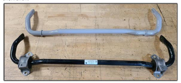
Lube the inside surface of the bushings with the supplied silicon grease. Install the bushings onto the bar as shown.
