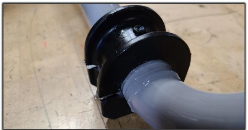
7F Install the included billet bushing brackets onto the bushings.
