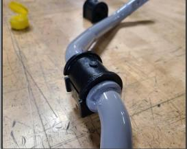
7R Install the aFe CONTROL sway bar in the same manner as factory removal.
