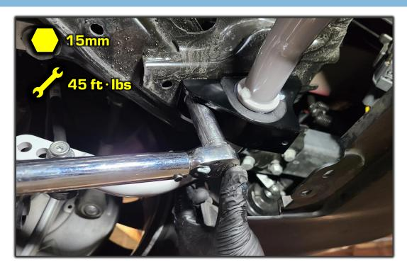
10F Fully tighten the factory nut onto the sway bar end. The hole furthest from the end is the stiffest setting. (Shown) The hole closest to the end is the softest setting. Tip: Add some thread locking compound to the end link stud to ensure long lasting tightness.
