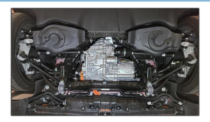
3R Unbolt the end link from the factory sway bar. Repeat on other side. Retain hardware for reinstallation.
