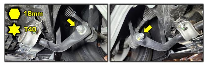
5F Unbolt the sway bar bushing mounts (4) nuts and remove the sway bar from the vehicle. Retain this hardware for reinstallation. Remove bar from vehicle.
