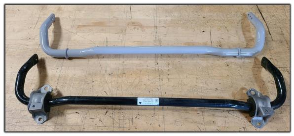
Lube the inside surface of the bushings with the supplied silicon grease. Install the bushings onto the bar as shown.
