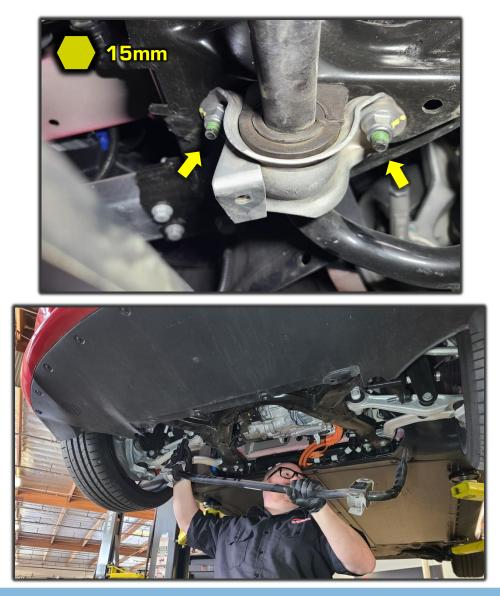
6F Lay out the factory sway bar with the aFe Control sway bar to match the orientation.
