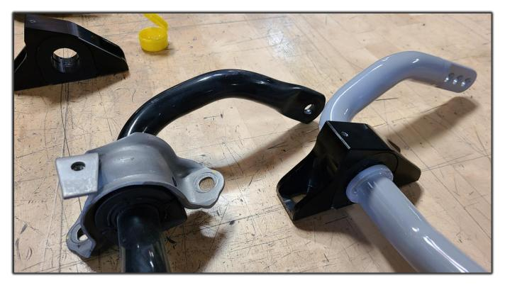
8F Reinstall the sway bar assembly back onto the vehicle in the same manner as removal. Attached the end links to the sway bar first to help with positioning the bar onto the car (do not tighten yet).
