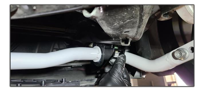
Adjust the bracket position so that the threaded hole in the forward position matching the under panel hole.
