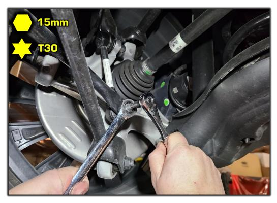
4R Unbolt the (2) bushing bracket bolts. Repeat on other side. Retain hardware for reinstallation.
