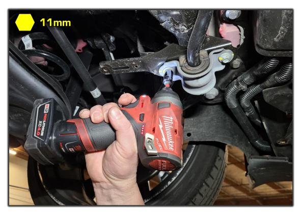
5R Remove the rear sway bar from the vehicle.
