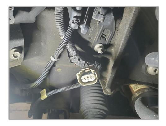
3. Plug in Ride Height Simulator. Make sure connector engages/locks back onto the Ride Height Simulator. Push red locking tab back into the connector to make sure it is locked.
