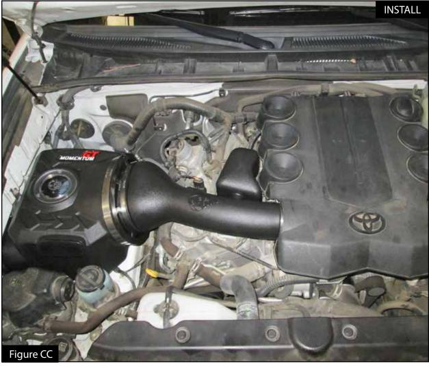
Refer to Figure CC for Step 41 Step 41: Reinstall the engine cover.
