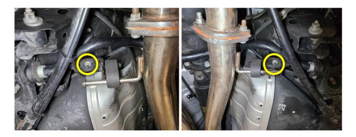
3R Unbolt the V-Brace using a 12mm socket. The brace does not need to be fully removed from the vehicle. It just needs to be able to drop out of the way to remove the sway bar.
