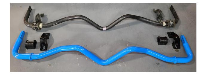
8R Grease the rear bushings with the supplied silicone lube and install the bushing onto the sway bar just outside of the centering rings.
