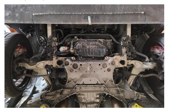
3F Disconnect the end links from the stock sway bar using a 19mm wrench for the stud and 17mm socket for the nut.
