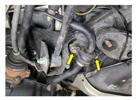
6R Remove the factory sway bar from the vehicle. Note the orientation of the sway bar when removing. (i.e. observe which is the top of the sway bar and how the ends are pointing.)
