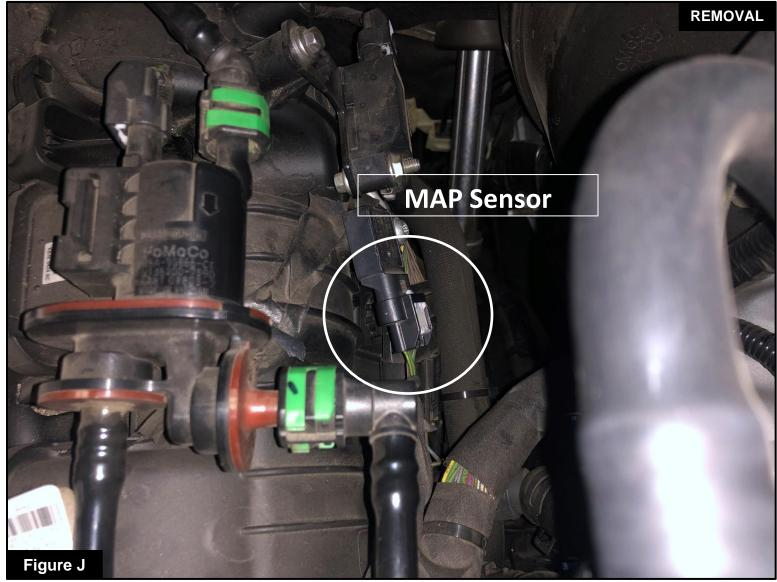
Refer to Figure J for Step 17 (Installation for Ranger Only)
