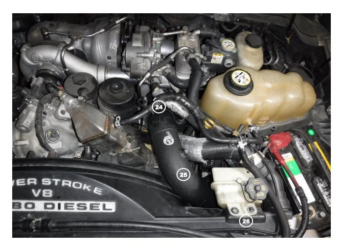
Note: Be sure to thoroughly clean all oil residue off of the connections before installing any of the aFe couplings onto the vehicle
