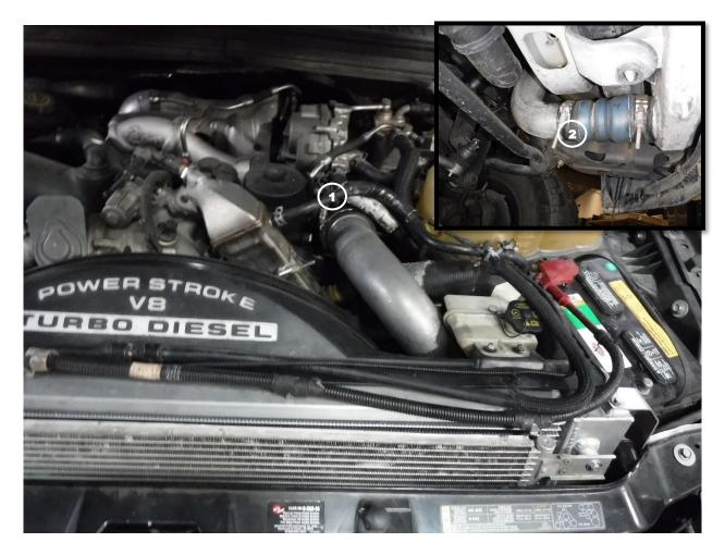
Note: it is recommended to remove the radiator from the vehicle in order to remove the factory hot side charge pipe for reuse later. The factory charge pipe can also be cut in half and removed from the vehicle if there are no plans for reusing it in the future.
