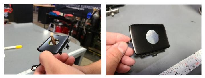
2. Test fit cap. Trim as needed until stem clears cap easily.
