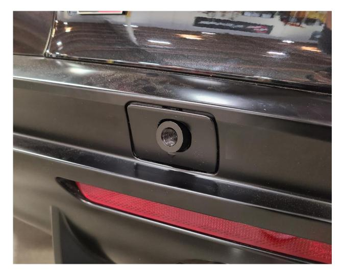
3. Thread in hook to the stem with the supplied bolt using a 15mm socket and firmly tighten it. You are now finished with the rear tow hook installation.
