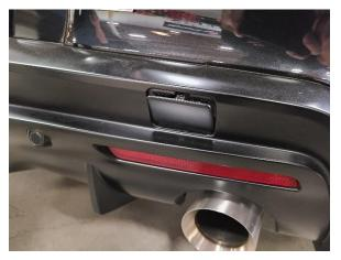
2. Remove cap once popped out. (*Note: gently pull on hanger to fully remove cap*)
