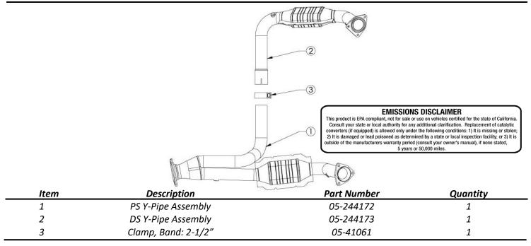
**aFe POWER recommends professional installation on this product.** Thoroughly inspect the aFe POWER exhaust system to make sure there is no damage from shipping (if damage is noted, immediately contact aFe POWER customer service). Allow time for your vehicle to cool down prior to installation. When working on your vehicle proceed with caution. Wear protective safety equipment; eye goggles and gloves to ensure a safe installation.
