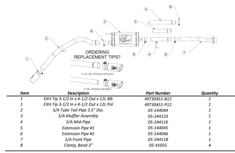
**aFe POWER recommends professional installation on this product.** Thoroughly inspect the aFe POWER exhaust system to make sure there is no damage from shipping (if damage is noted, immediately contact aFe POWER customer service). Allow time for your vehicle to cool down prior to installation. When working on your vehicle proceed with caution. Wear protective safety equipment; eye goggles and gloves to ensure a safe installation.
