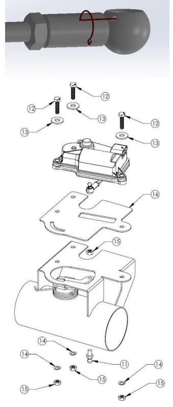
26. Remove the locking wire securing the front exhaust valve linkages to the exhaust valve with a pick or small screwdriver (See Image). Retain for later use.
