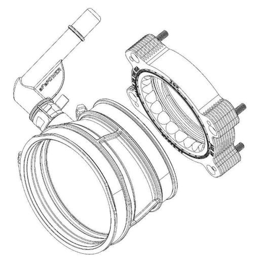
advanced FLOW engineeringSilver Bullet Throttle Body SpacerInstruction ManualP/N: 46-34017B (Fits with Factory Air Intake)Make: CHEVROLETModel: CORVETTE (C8)Year: 2020-2023Engine: V8-6.2L
