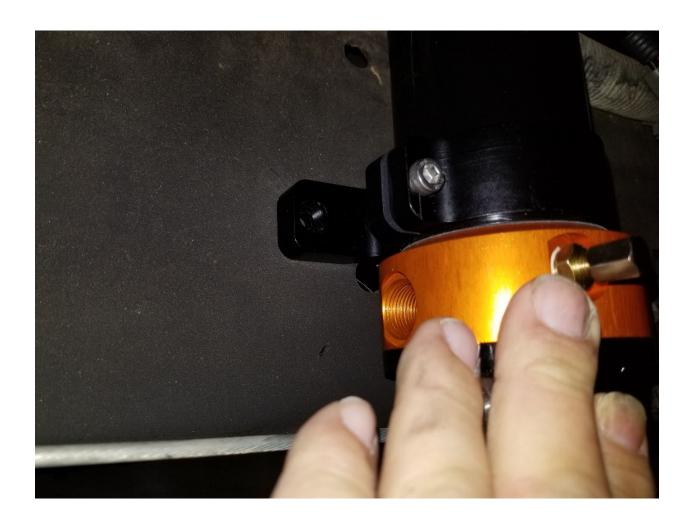
2. Find a suitable location for the fuel pump assembly and mark the two (2) holes using the billet aluminum mounting bracket as a guide.
