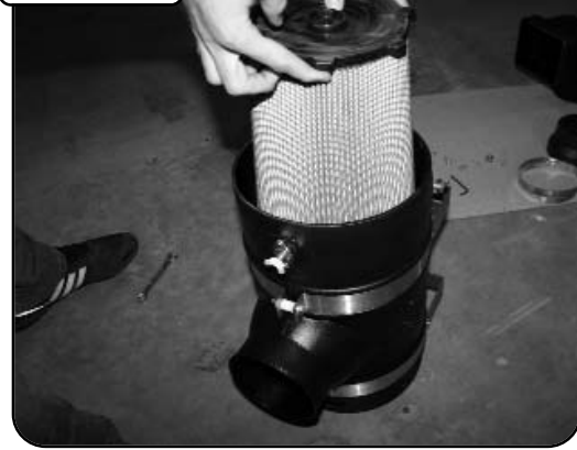
Install filter into canister and tighten using 5/16" nut driver. (Use cut out slots to tighten.)
