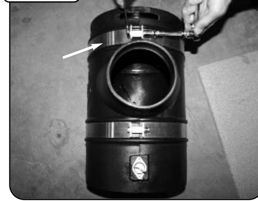
With 10mm socket or wrench, tighten down band clamps with hardware provided. Use 1 flat, 1 lock washer per screw (Make sure nylon spacer is between clamp to keep from collapsing.)
