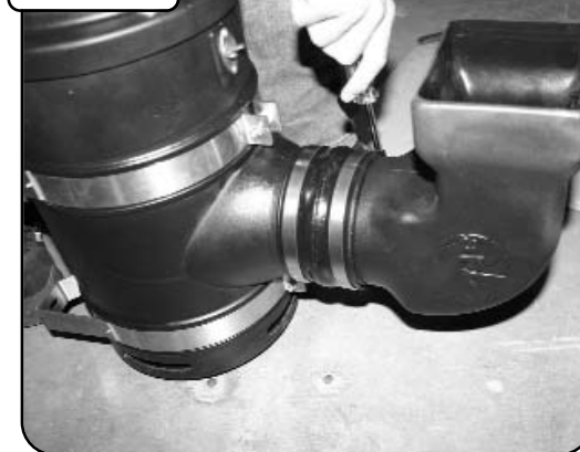
Install your snorkel with hump coupler and clamps and tighten. (Snorkel and band clamps can be adjusted)
