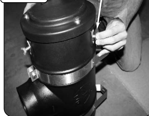
Line up cover clips to Dzus fasteners and secure cover.
