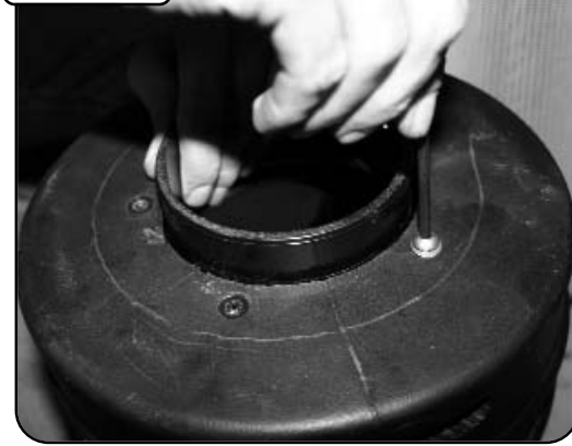
Install button head screws and wavy washers through canister with 5-1/2" adapter.
