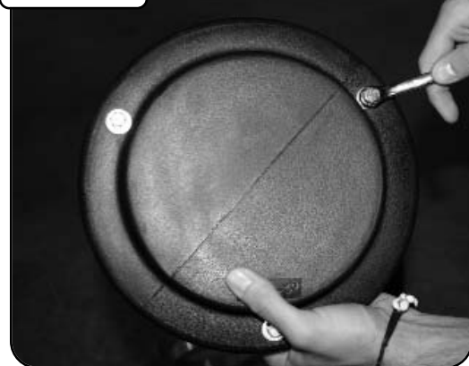
Install cover clip with hardware provided, and tighten using 10mm socket or wrench.
