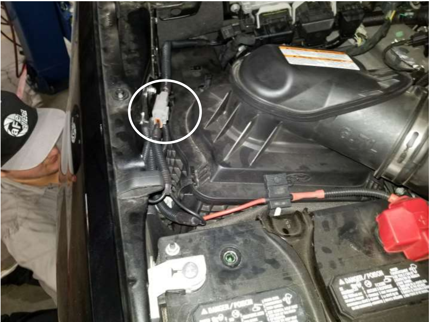
32. Plug the supplied relay harness into the weatherproof connector on the power harness.
