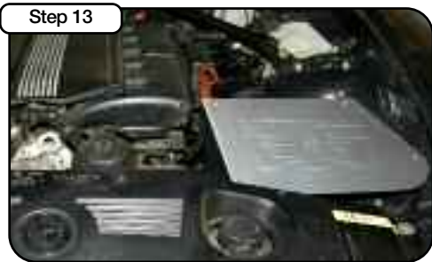
Your installation is now complete. Tighten all connections and clamps. Re-connect negative battery terminal. Re-check after a few hours.
