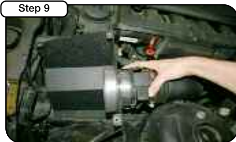
Lower housing into the engine bay. Fasten the MAF sensor to the housing and secure with the two spring clips.
