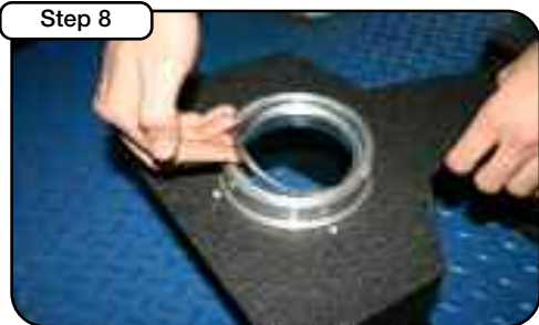
Carefully place the rubber MAF sensor gasket into the slot inside the air filter adaptor.
