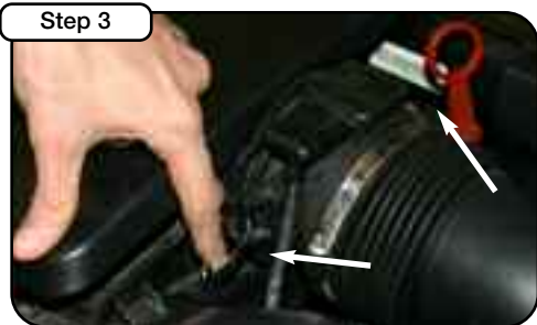
Disconnect negative terminal from battery. Loosen the hose clamp on the intake tube. Disconnect the two metal clips on the side of the MAF sensor.
