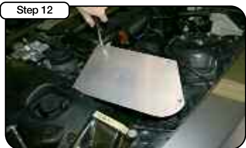
Place aluminum cover over housing. Secure with the four remaining button head screws.
