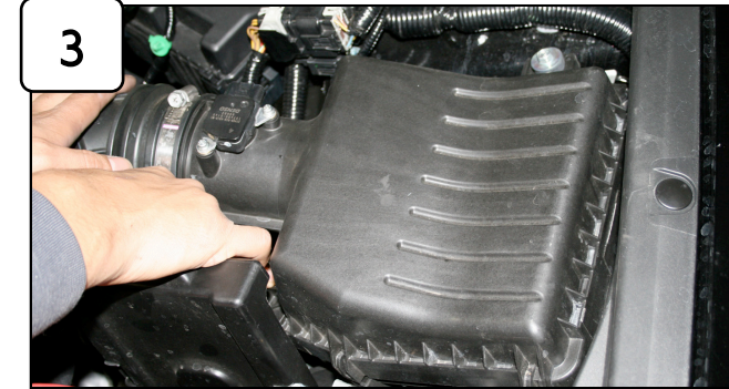
3 Disconnect MAF sensor harness. Unclip upper half of air box. Loosen clamps using 10mm socket or wrench. Pull crank case line away from tube. Remove upper half of stock intake.
