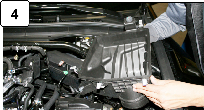
4 With 10mm socket or wrench loosen the bolt securing the bottom half of the air box and remove.
