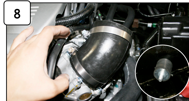
8 Install elbow coupler to throttle body and position using clamps provided. Do not tighten. Install isolation mount to threaded hole on inside of engine compartment.
