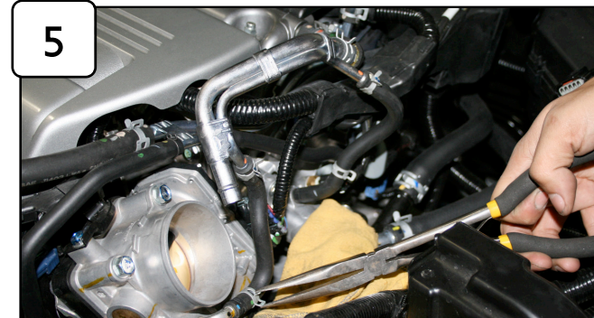
5 Remove crank case line attached with throttle body coolant line. Have a shop towel or rag handy to catch any leaking coolant. Use pliers to remove both lines. Save small clamps for later install. Caution: Coolant may leak from line when removing!
