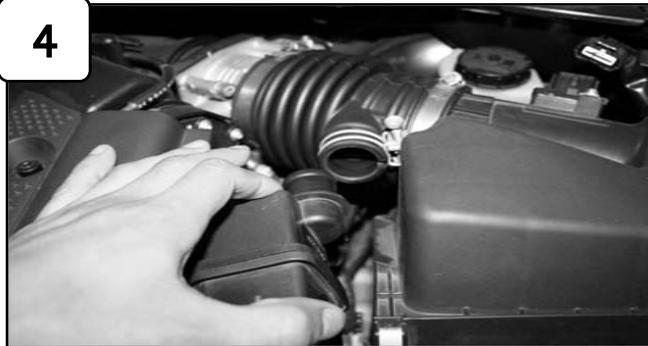
With 10mm socket or wrench loosen crank case line. Disconnect MAF sensor harness.
