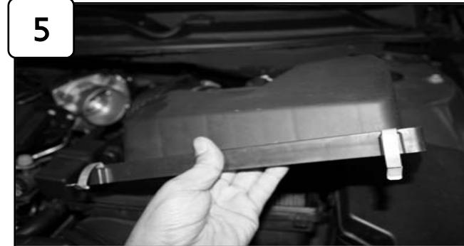
Remove upper half of air box and stock tube assembly.
