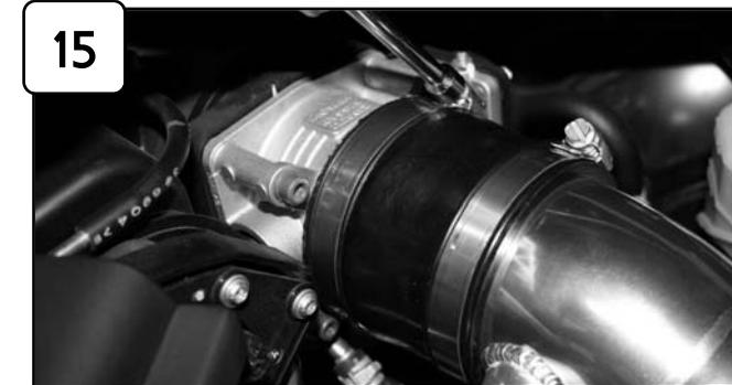
15 Tighten all clamps using 5/16" nut driver.
