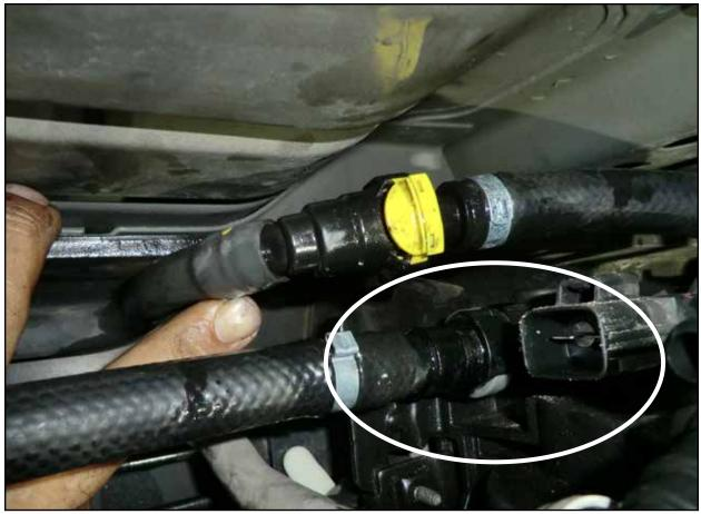
• Install the straight female quick disconnect fitting on the supplied fuel outlet hose (black 90° -8 AN fitting - shown below) onto the male side of the stock fuel pump.
