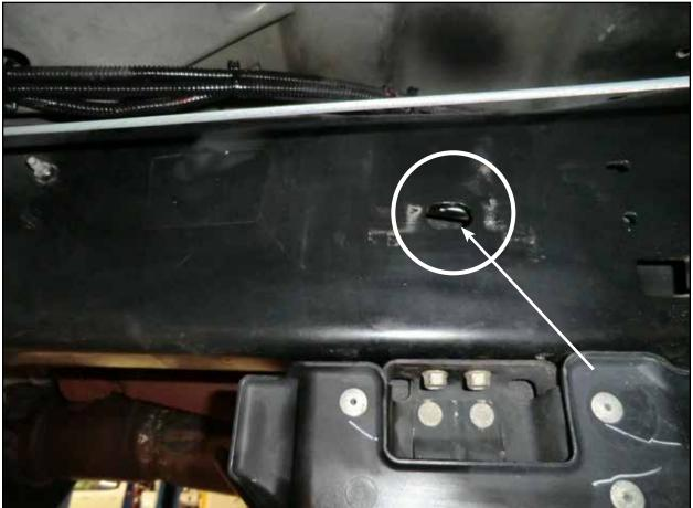
• On the driver's side of the truck, under the rear door, you will see an oval hole. Use this hole to mount the supplied carbon steel frame bracket to the frame
