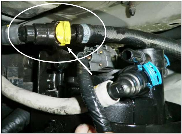
• Install the straight male quick disconnect fitting on the supplied fuel inlet hose (silver 90° -8 AN fitting shown below) into the female side of the stock fuel feed line.
