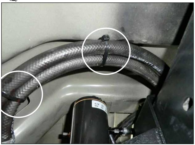
• Using the supplied nylon cable ties, secure the new hoses (as shown above).
