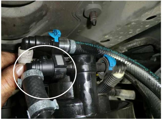
• Install the 90° female quick disconnect fitting on the fuel return line (as shown below) onto the male connection of the stock fuel pump.
