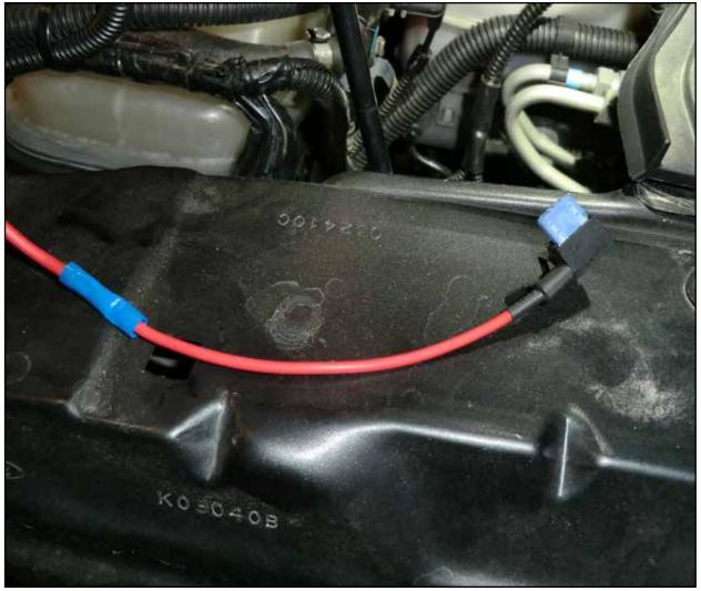
• Attach the power wire from the relay harness to the supplied add a harness fuse adapter.
