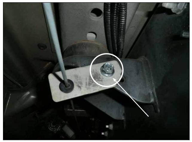
• Remove the bolt holding the parking brake cable guide from the truck.
