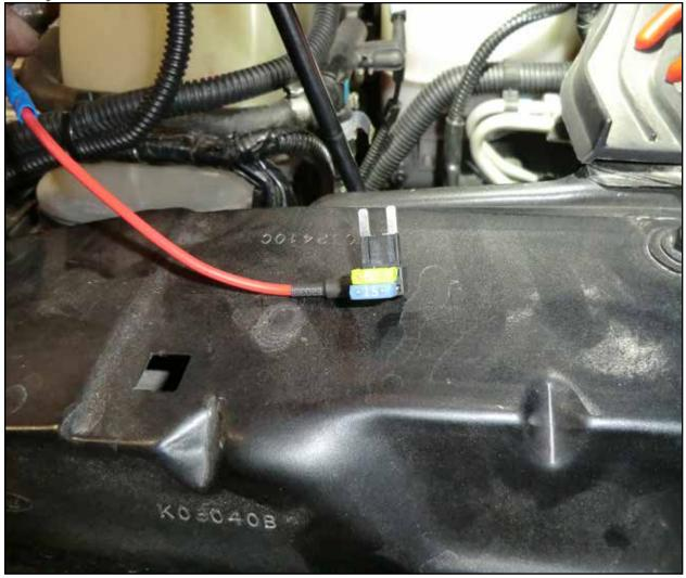
• Install the fuse removed on page 32 into the open location on the add a harness fuse adapter (not in line with the wire).
