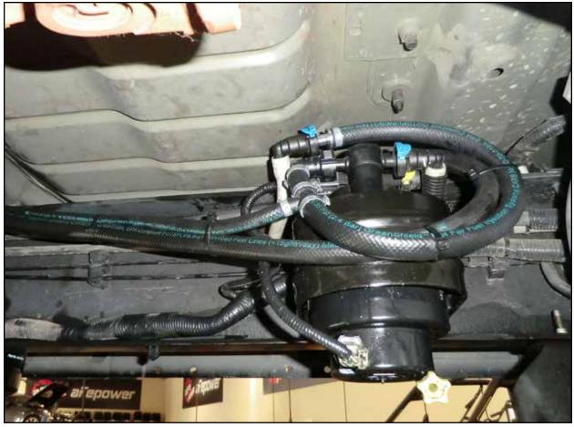
**Note:** This is what the connections at the fuel pump should look like after all the supplied hoses are connected.
