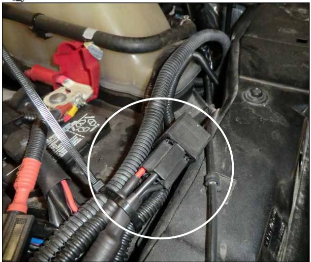
• Secure the relay harness using a supplied nylon cable tie.
