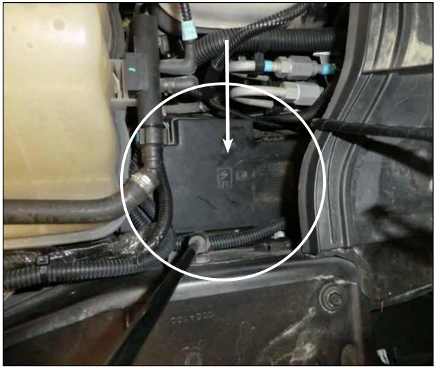
• Locate the fuse box in the engine compartment (located on the driver's side rear corner next to the master cylinder, behind the engine coolant tank).
