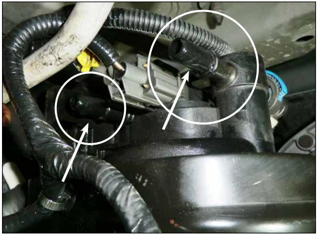
• Disconnect the fuel supply and the fuel return line.
