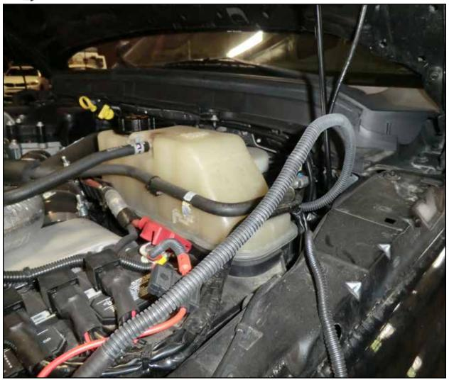
• Run the other end of the power harness along the inside of the frame into the engine compartment.
