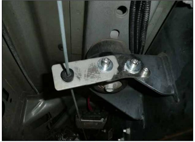
• Install the supplied parking brake cable bracket with the supplied hardware and tighten.
