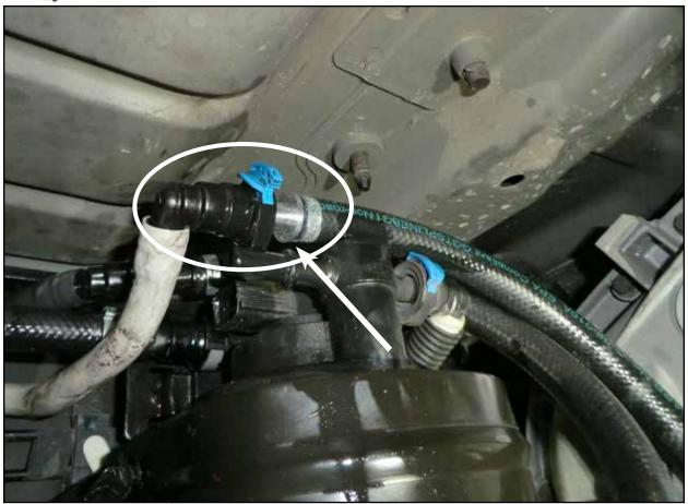
• Install the straight male quick disconnect fitting on the supplied fuel return line (as shown below) into the female side of the stock fuel return line.
