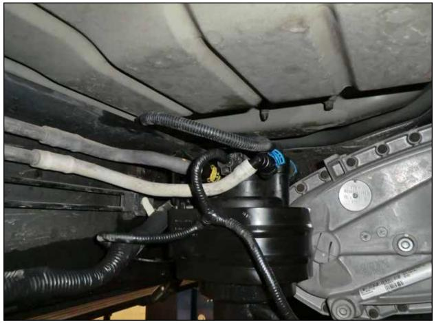
• Clean the area around the stock fuel pump (located on the driver's side, inside the frame) to prevent dirt and debris from going into the lines.
