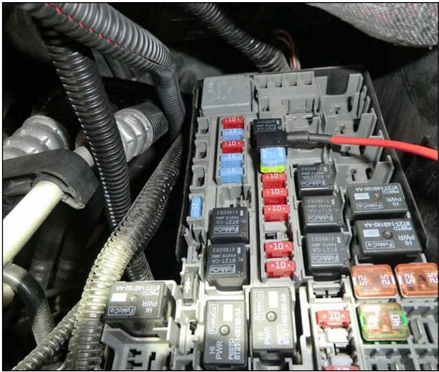
• Install the add a harness fuse adapter (with installed fuses) into the 12-volt source location chosen on page 32.
