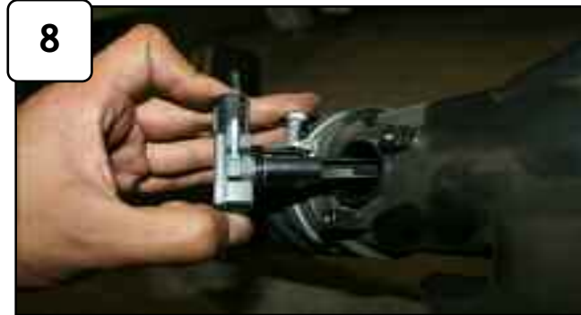
Remove MAF sensor using phillips screwdriver.
