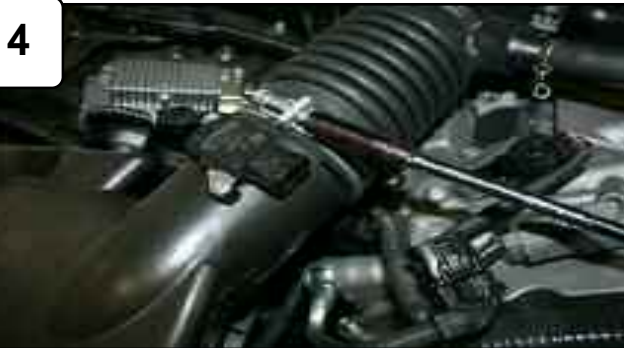
With 10mm socket and ratchet, loosen the two clamps using a 10mm socket or wrench from the OEM intake tube and airbox. Disconnect MAF sensor harness.
