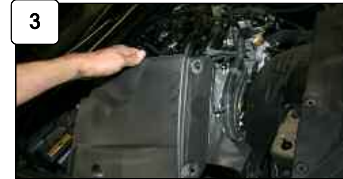
Remove engine cover and front/passenger plastic covers.
