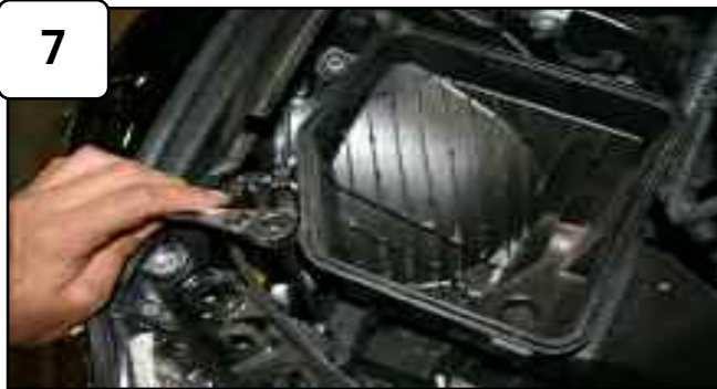
With 10mm socket or wrench loosen the 2 bolts holding in bottom half of air box and remove.
