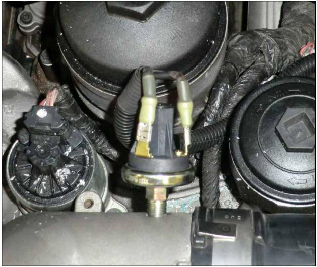
• Connect the supplied pressure switch harness to the pressure switch (either wire can be attached to either terminal).
