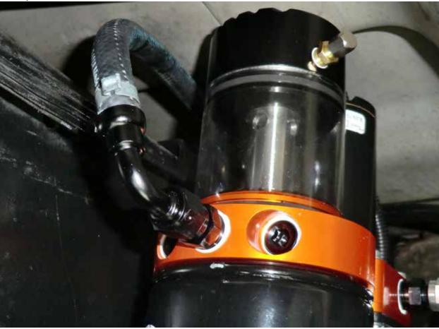
• Install the fuel outlet hose (black 90° -6 AN fitting) onto the male -6 AN fitting on the fuel outlet port of the fuel manifold assembly.
