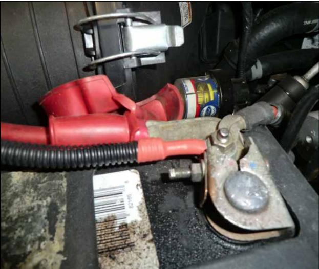
• Connect the red wire ring terminal on the power harness to the positive side of the battery.
