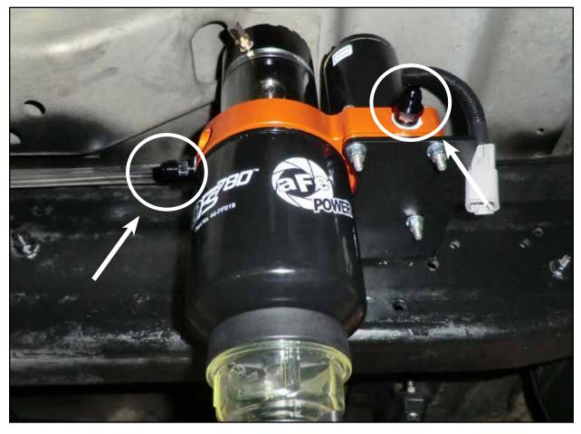
• Install the 2 x 3/8" NPT to -6 AN fittings into the fuel manifold assembly (as shown above).
