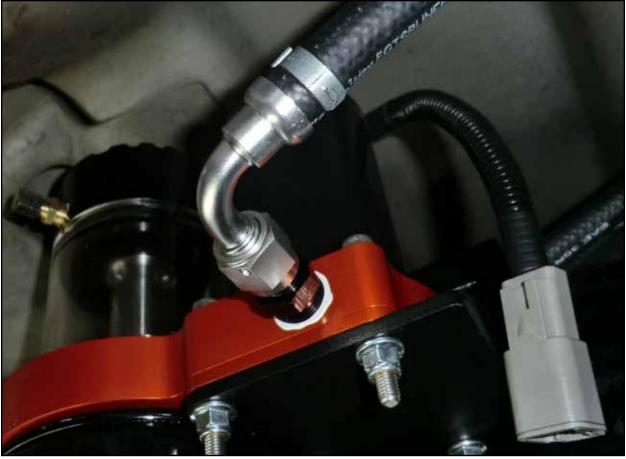
• Install the fuel inlet hose (silver 90° -6 AN fitting) onto the male -6 AN fitting on the fuel inlet port of the fuel manifold assembly.
