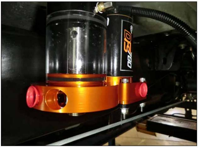
• Mount the supplied fuel manifold assembly to the supplied carbon steel frame bracket using the supplied hardware and tighten.
