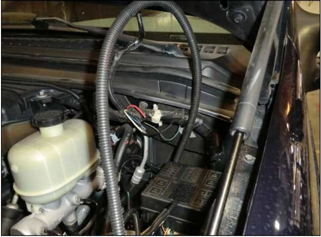
• Run the other end of the power harness along the frame into the engine compartment.
