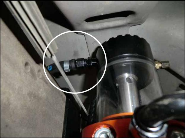
• Install the fuel return hose (-4 AN fitting) onto male -4 AN fitting on the top of the sight glass cover.
