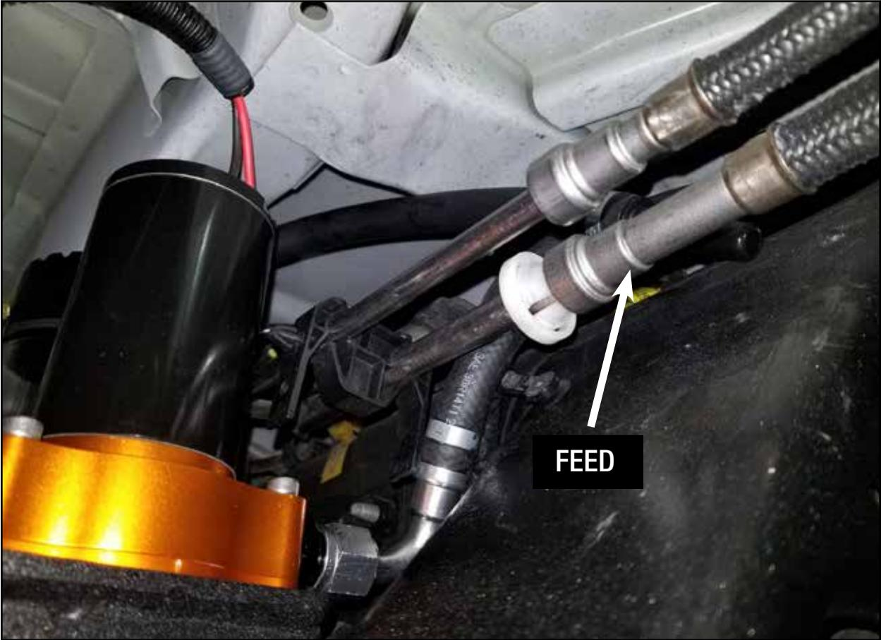
**Step 14:** Disconnect the factory fuel feed line using a quick disconnect tool.
