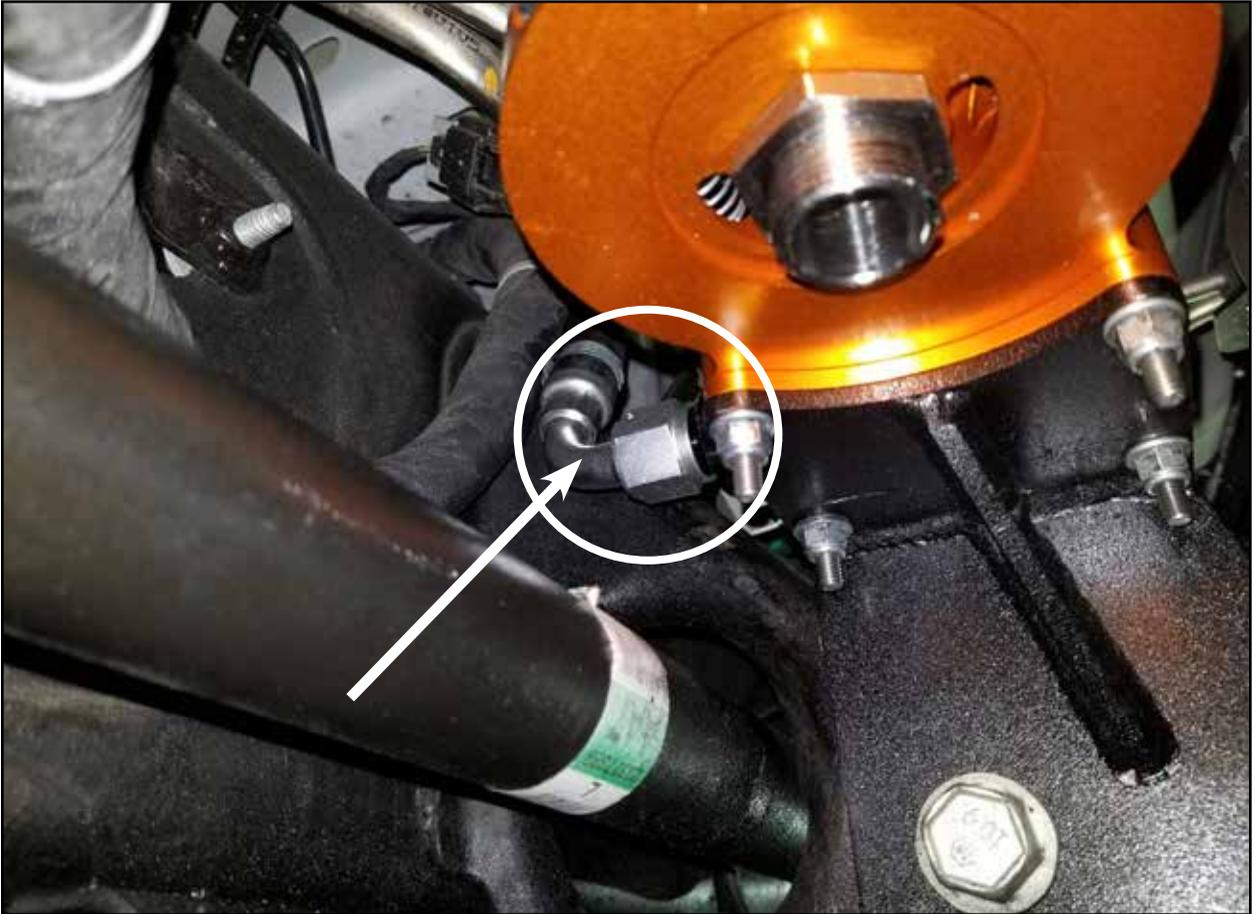
**Step 12:** Install the fuel inlet hose (silver 90° -8 AN fitting) onto the male -8 AN fitting on the fuel inlet port of the fuel manifold assembly.
