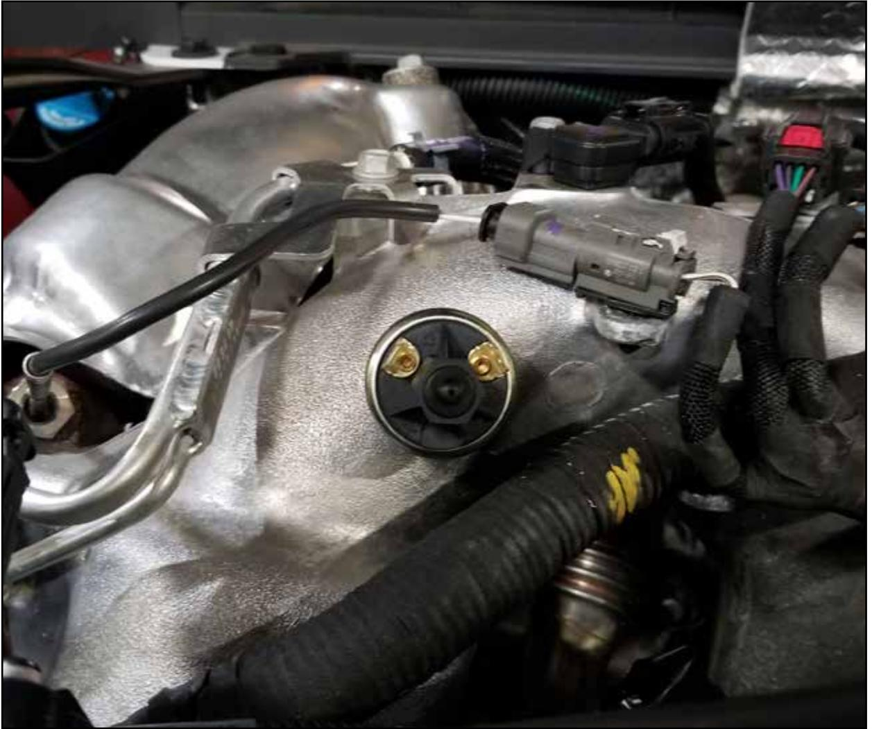
**Step 34:** Install the supplied pressure switch into the intake manifold (1/8" NPT).
