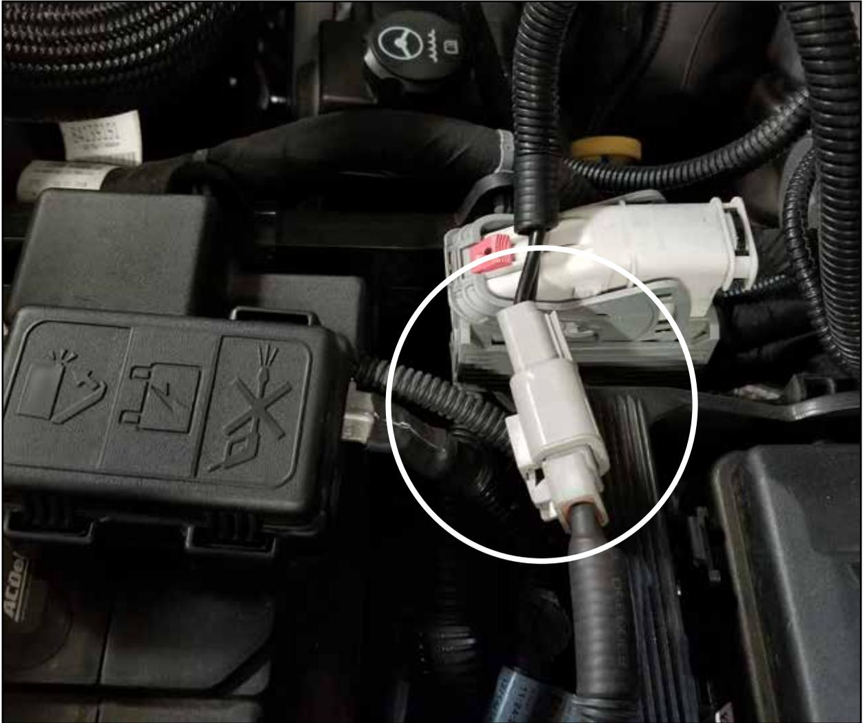
**Step 38:** Plug the pressure switch harness onto the Deutsch connector on the power harness.
