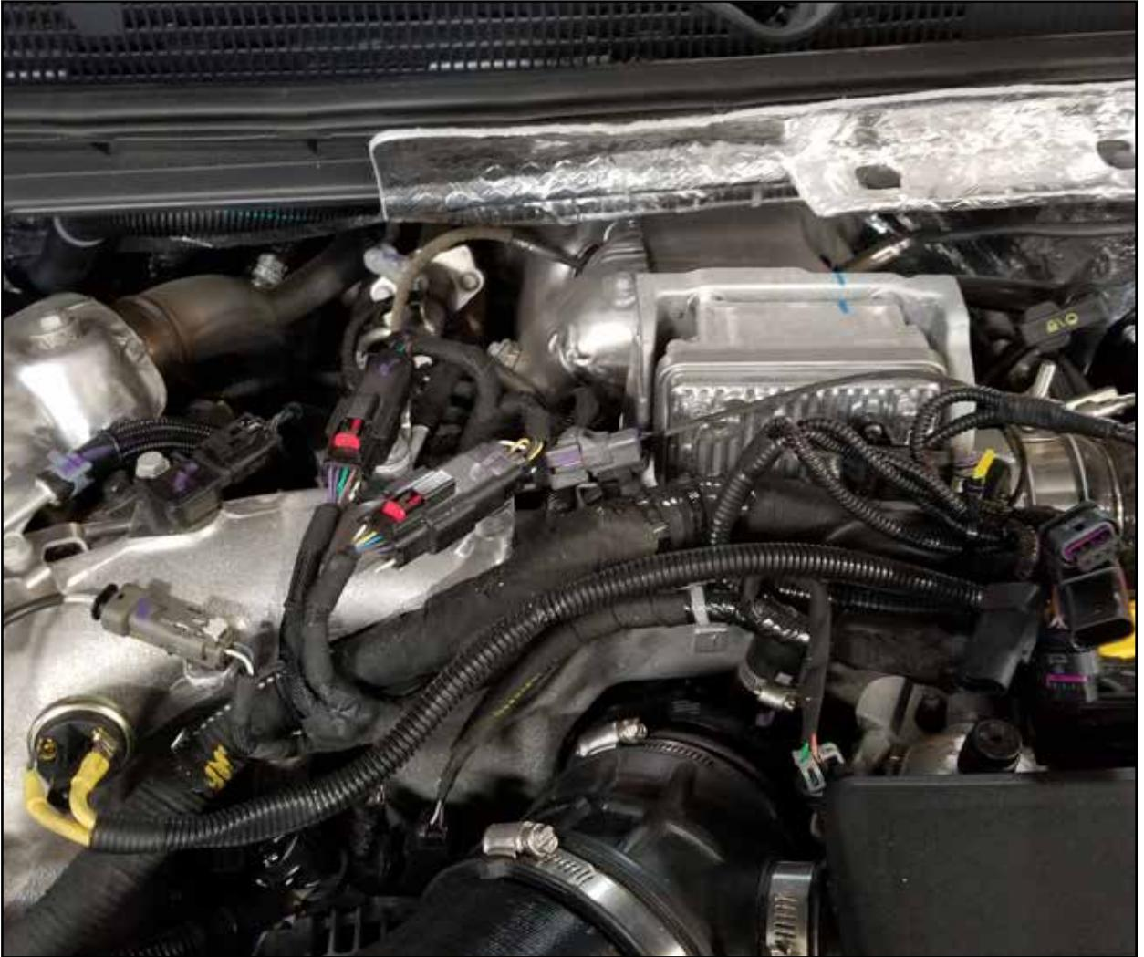
**Step 35:** Connect the supplied pressure switch harness to the pressure switch (either wire can be attached to either terminal).
