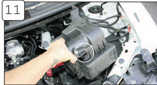
11 Pull up on the stock intake box and it will come out. After the box is removed, unscrew the MAS sensor and remove it from the stock box. After removing stock air box re-install battery and stock resonator.
