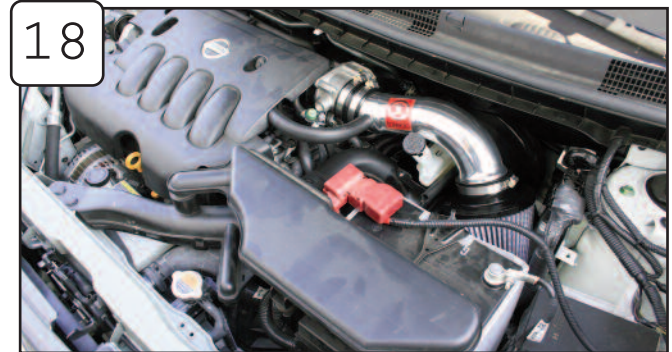
18 The installation of your Takeda performance intake is now complete. Place the included CARB EO sticker on or near the intake system on a smooth, clean surface. E.O. identification label is required in passing the smog inspection.
