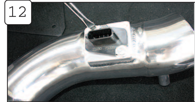
12 Install the MAS flow sensor into the takeda tube using the supplied screws.
