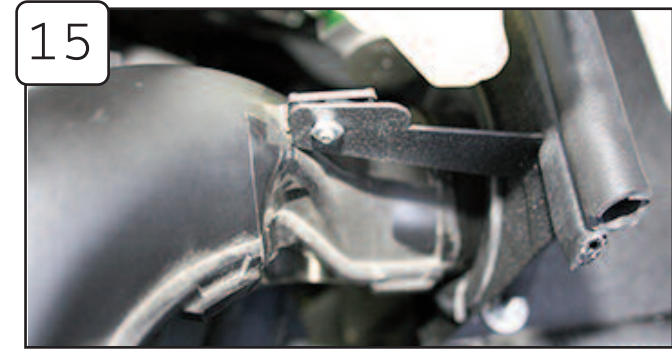
15 Re-insert stock ram air tube into the opening in the heat shield. Using the supplied hardware, mount the housing and ram air tube together.
