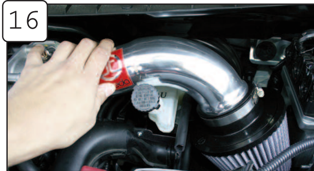
16 Install the coupling and filter onto the intake tube using a 5/16" nut driver. Position the intake tube into the vehicle making sure to leave clearance from the fluid reservoir. Note: Under acceleration the intake tube will be pulled toward the firewall a inch or two. Leave clearance for this.
