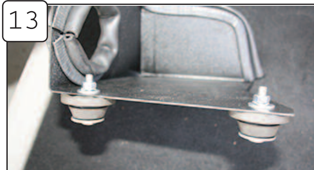
13 Using the stock rubber mounts that hold the stock air box down, install the following bolts with supplied washers and nuts with spacers as seen in the photo. Note: Make sure spacer is in between grommet to prevent collapsing.
