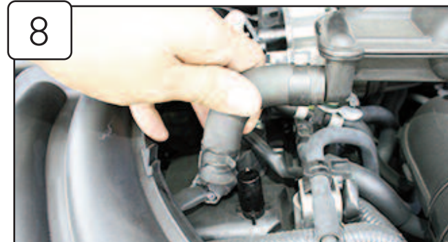
Disconnect the crank case vent line with pliers.
