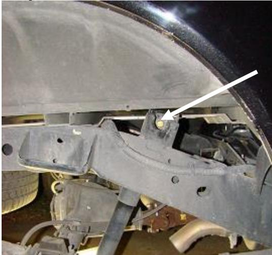
6. Using the stock nuts and bolts, install your new shocks with the top eyelet first and the bottom eyelet second.
