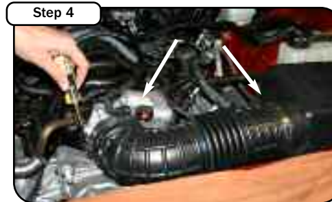
Loosen the two hose clamps on the intake duct and remove duct from engine bay.
