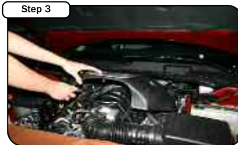
Disconnect negative terminal from battery. Lift off Hemi engine cover. Remove the Temp. Sensor on the side of the intake duct. Be careful not to damage sensor
