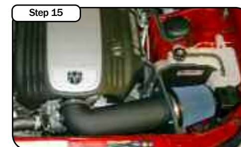
Your installation is now complete. Tighten all connections and clamps. Re-check after a few hours. Place the included CARB EO Sticker on or near the intake system on a smooth, clean surface. E.O identification label is required in passing the Smog Check Inspection.
