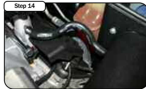
On SRT-8 models re-use factory crank case breather hose (shown in above photo). On non SRT-8 models use provided hose and clamps. Replace cover and reconnect battery.
