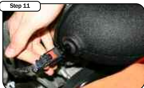
Insert the rubber grommet into the side of the intake duct and re-connect the Temperature Sensor.
