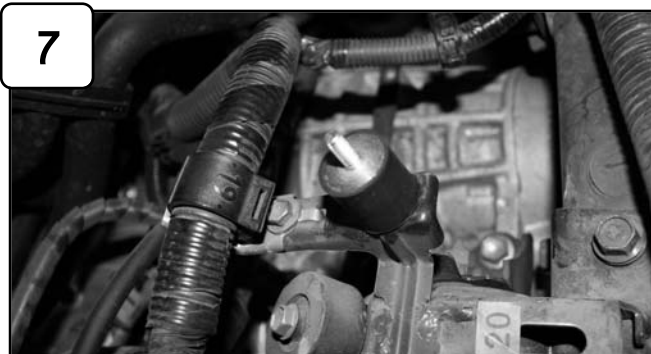
Install M6 isolation mount to air box bracket.
