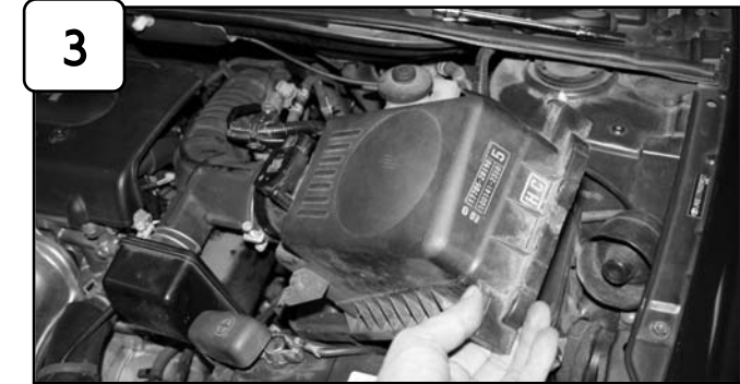
Disconnect MAF sensor and loosen clamp using 10mm socket or wrench. Unclip upper half of air box and remove. With phillips screwdriver loosen VSV module from tube. Loosen clamp with pliers on throttle body and remove stock intake tube.
