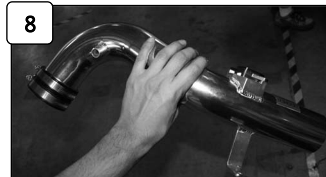
Install upper intake tube assembly into vehicle with provided 05-00417 coupling and clamps. Do not tighten.
