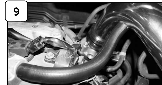
Remove engine cover using 10mm socket or wrench. Remove stock crank case line and replace with provided 5/8" hose. Re-install engine cover and tighten.
