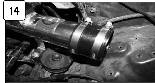
14 Attach 05-00418 coupling with clamps to upper intake tube assembly. Do not tighten.
