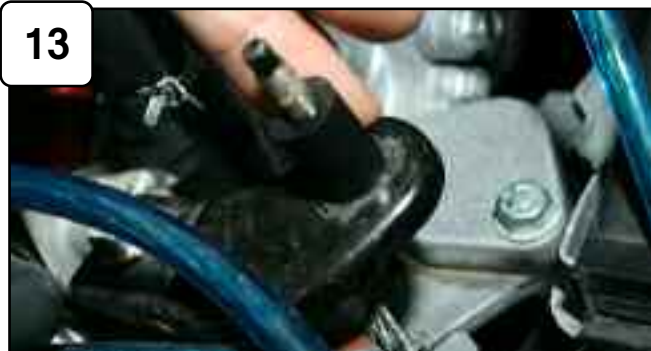
With provided nylon spacer, place on air box mounting point.
