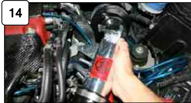
Install intake into vehicle and position tab to mounting point and coupler.
