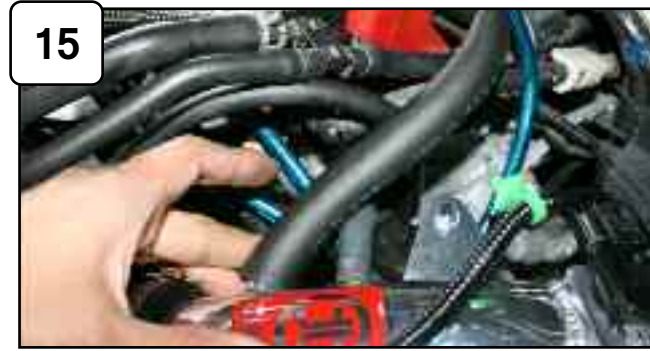
Reinstall the crank case line using the 5/8" hose provided. Re-install vacuum line to new intake tube.
