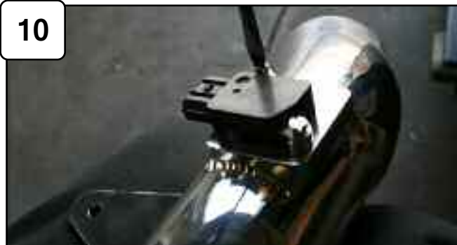
Install MAF sensor to intake tube using new M4 screws provided.
