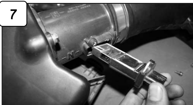
7 Remove MAF sensor from stock air box using T20 torx bit.
