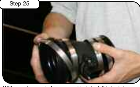
Step 25 With couplers and clamps provided, install tube into vehicle.
