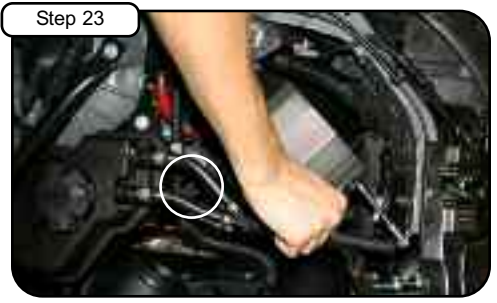
Step 23 Re-install nut from step 4 and tighten using 10mm socket or wrench.
