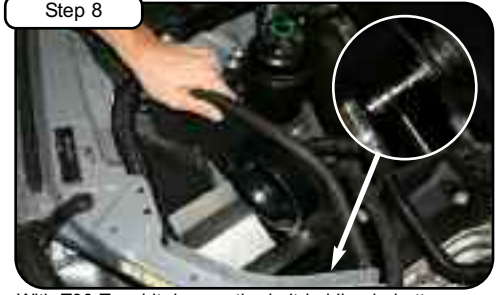
Step 8 With T30 Torx bit, loosen the bolt holding in bottom ram air unit. Place housing into vehicle. Attach tab to housing to ram air unit. Re-install bolt and tighten.
