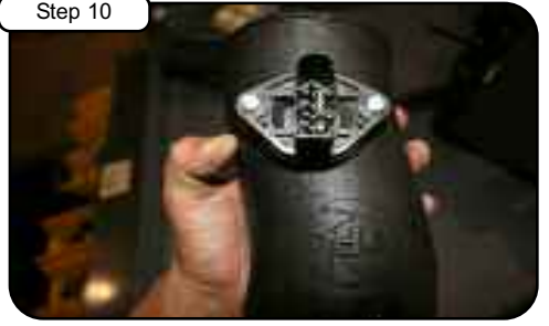
Step 10 Remove MAF sensor from airbox and install into new tube (05-00889) with screws and gasket provided. Tighten using flathead screwdriver.
