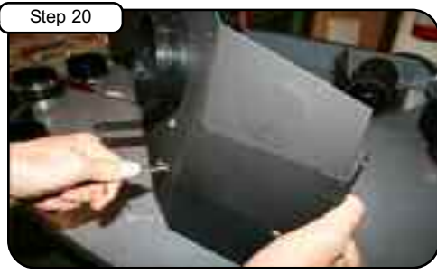
Step 20 Attach filter adaptor to housing using 3 button head screws & wavy washers. Tighten using 5mm allen key.
