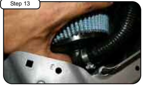
Step 13 Install filter on adaptor. Install plastic elbow with mini clamp provided to filter and smog pump line from step 12. Tighten mini clamp using 1/4" nut driver.
