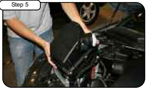
Step 5 Remove air box from vehicle.
