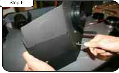
Step 6 Attach filter adaptor to housing using 3 button head screws & wavy washers. Tighten using 5mm allen key.
