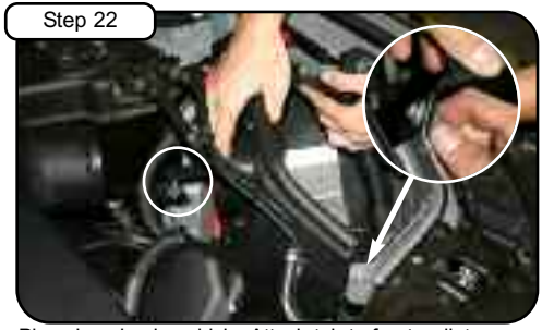
Step 22 Place housing in vehicle. Attach tab to front radiator support using supplied M6 screw and washer.
