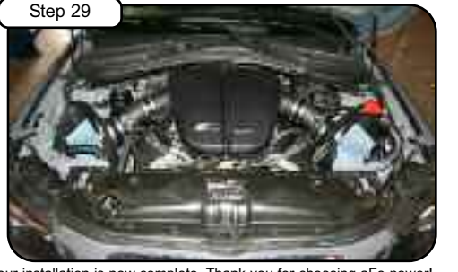
Step 29 Your installation is now complete. Thank you for choosing aFe power! NOTE: Place enclosed CARB EO sticker on a clean/smooth surface on or near the intake system. EO identification label is required in passing the Smog Check inspection. Retighten all connections after approximately 100-200 miles.
