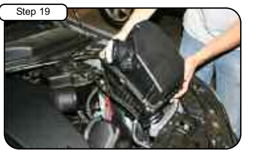
Step 19 Remove air box from vehicle.
