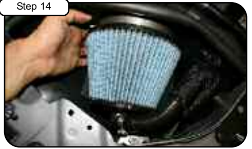
Step 14 Position smog pump line above ram air unit. Tighten clamp on filter using 5/16" nut driver. Re-connect MAF sensor harness. Continue to page 2 for driver side installation.
