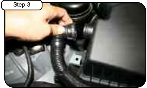
Step 3 Disconnect smog line from air box.
