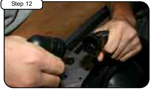
Step 12 Remove plastic smog pump elbow. Note: If difficult to remove, a heat gun may allow for elbow fitting to come out easier.
