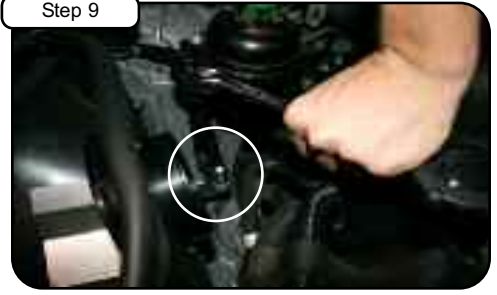
Step 9 Re-install nut from step 4 and tighten using 10mm socket or wrench.
