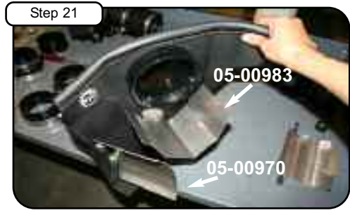
Step 21 Attach air diverters to housing using button head and wavy washers. Tighten using 5mm allen key. Install 3/4" trim seal on housing. Install small 7/16" trim seal to corner of housing. Note: Failure to install air diverters may result in CEL (Check Engine Light).
