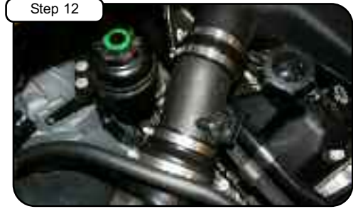
Step 12 Position tube and tighten using 5/16" nut driver.
