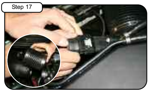
Step 17 Disconnect MAF sensor harness. Loosen clamps with 1/4" nut driver. Take out plastic intake tube.
