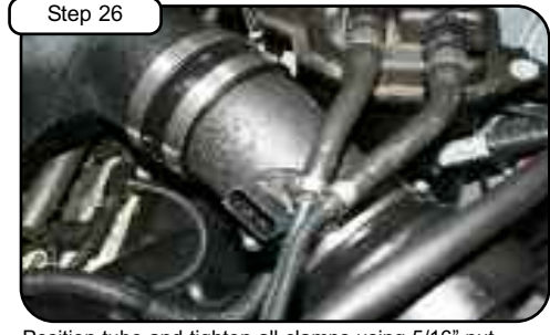
Step 26 Position tube and tighten all clamps using 5/16" nut driver.
