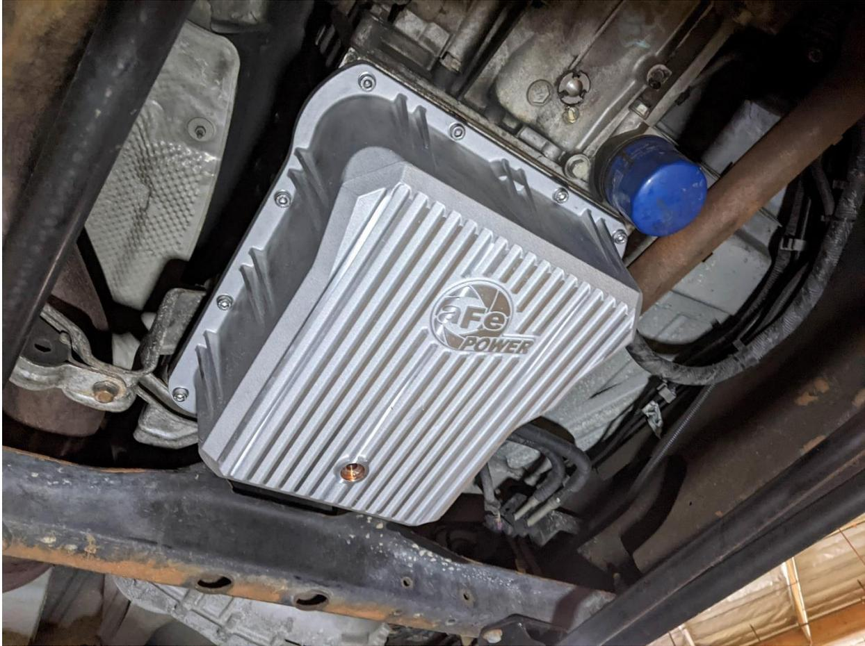
18. Hold the transmission pan up into position, aligning the screw holes. Install four (4) M8x1.25x30 socket head screws and M8 flat washers into each of the corners to hold the pan into position.
