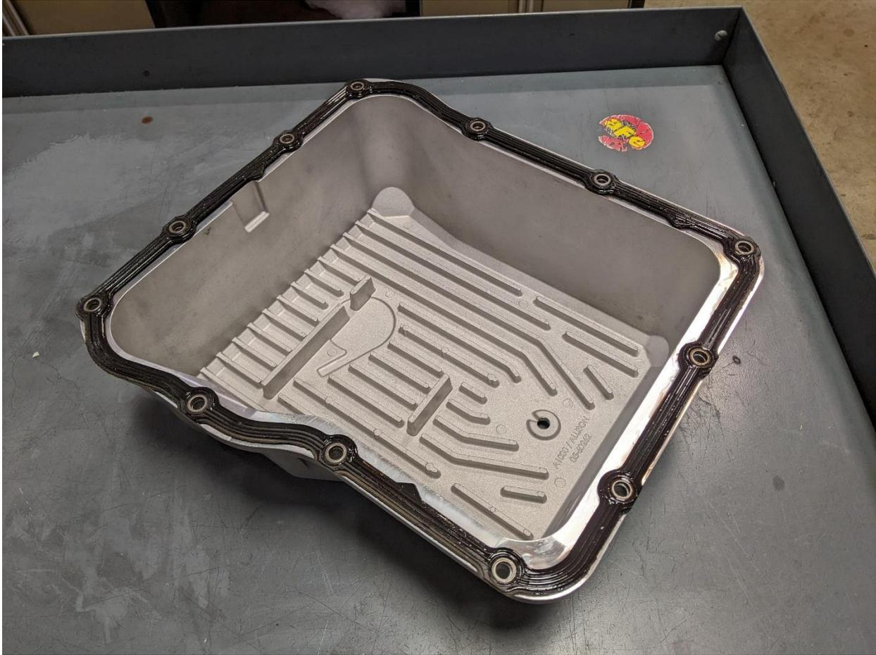
15. Hold the supplied aFe transmission pan up to the gasket surface to make sure you will be able to maneuver it into place.
