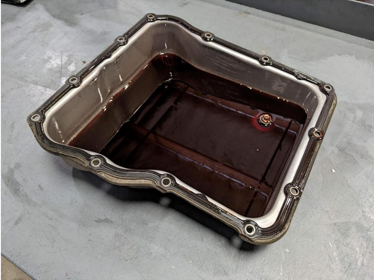
6. Remove eight (8) of the 12 screws holding up the pan, leaving one in each corner.
