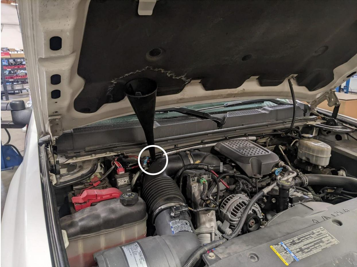
**Note: The truck needs to be warmed up, running, and in neutral in order to get an accurate reading on the dipstick. Periodically check the dipstick reading while filling to prevent overfilling.**
