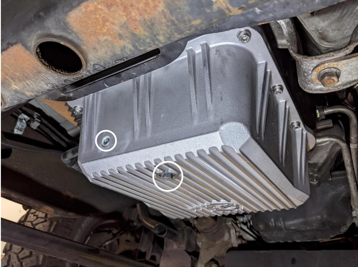
21. Install the supplied M12x1.25 magnetic drain plug and crush washer (secure about ½ turn past finger tight).
