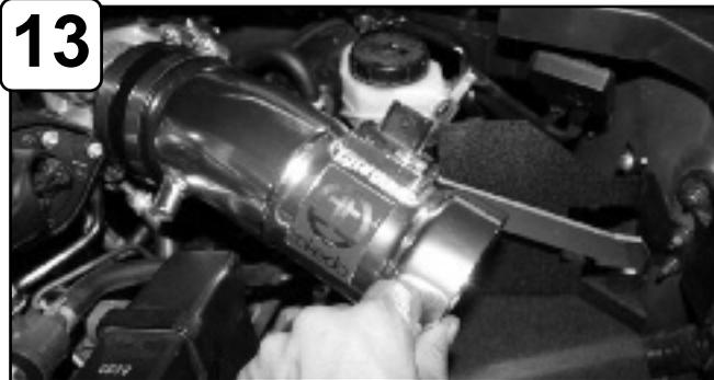
13 Install intake tube assembly and position tab to isolation mount. Do not tighten.
