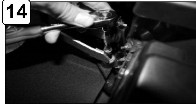
14 Tighten intake bracket using provided flat washer, wavy washer and nut.
