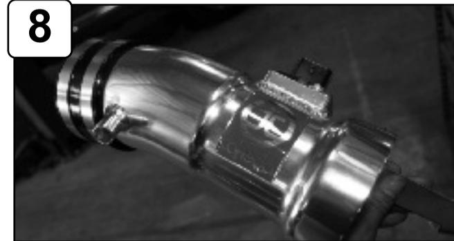
With provided M4 screws, install MAF sensor to new intake tube. Attach coupler to tube with clamps provided. Do not tighten.
