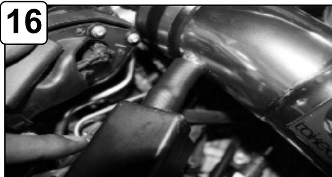
16 Attach 5/8" hose from the crank case port on the intake to the stock plastic vacuum port. Re-connect MAF sensor harness.
