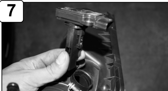
With t20 torx bit screwdriver remove MAF sensor from air box.
