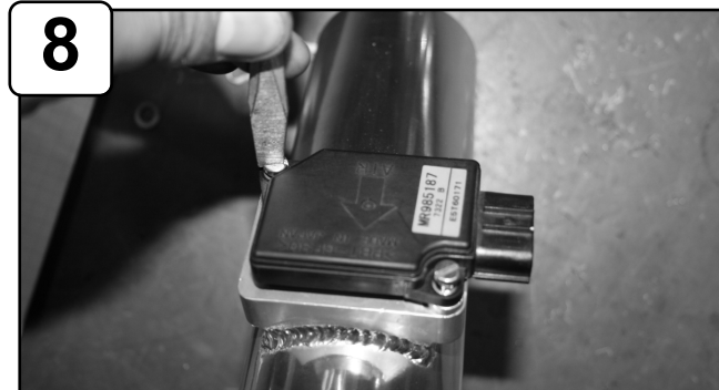
Install MAF sensor to new tube and secure using M4 screws provided.
