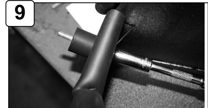
Tighten isolation mount provided on housing using 10mm socket or wrench.
