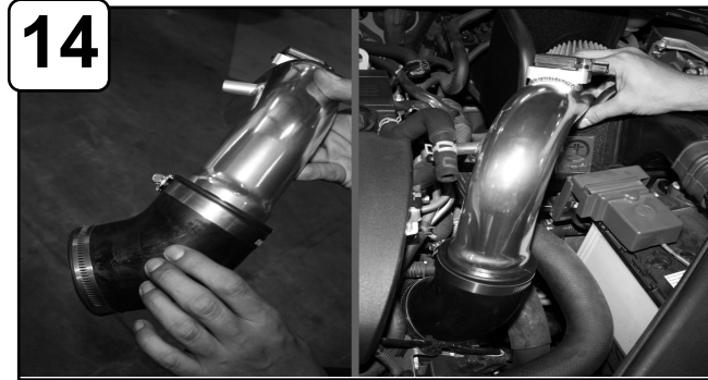
14 Attach elbow coupling with clamps to tube. Position tube to throttle body and tab on tube to isolation mount.
