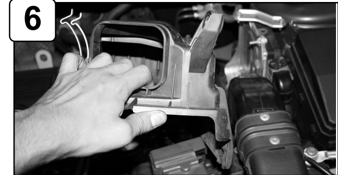
Pull back ram air assembly from air box and remove.
