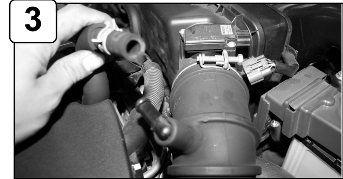
Disconnect MAF sensor and pull back crank case line and remove from engine.
