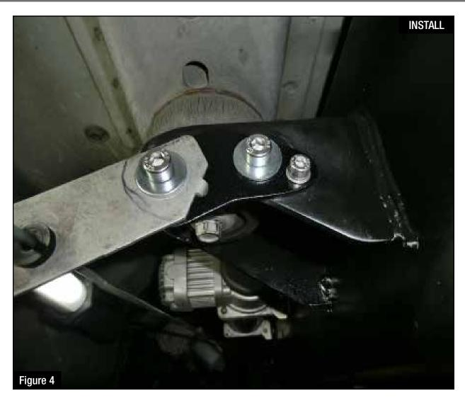
Step 5: Install the new relocation tab for the emergency brake with the supplied hardware and tighten
