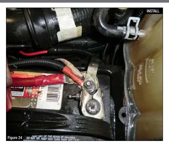
Step 27: Connect the red wire ring terminal to the positive side of the battery.
