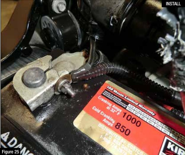
Step 28: Connect the black wire ring terminal to the negative side on the battery.
