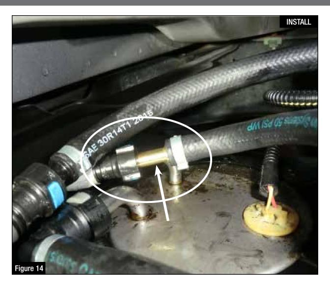
Step 16: Install the supplied fuel return line to the female side of the stock return fuel line (as shown below).
