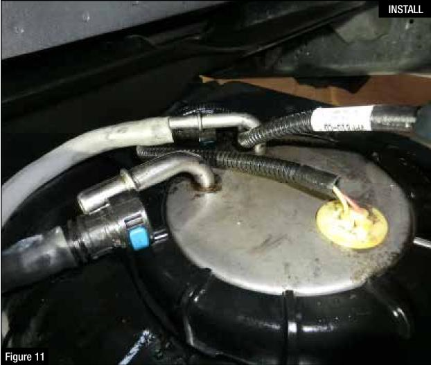
Step 13: Disconnect the fuel supply and the fuel return lines.
