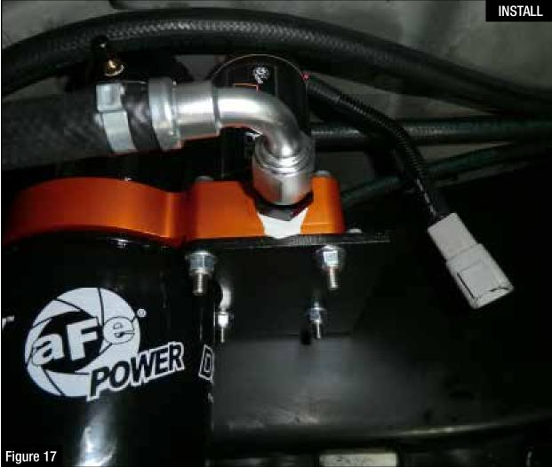
Step 18: Install the fuel inlet hose (90° silver "AN" fitting) onto the fuel inlet port of the DFS780.
