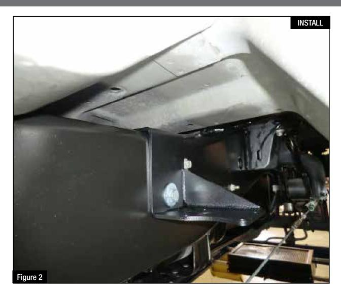
**Step 3:** Mount the supplied bracket to the frame using the supplied  $\frac{1}{2}$ "-13 x 1.50" bolt, two (2)  $\frac{1}{2}$ " washers &  $\frac{1}{2}$ "-13 lock nut.
