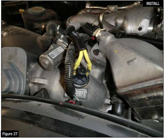
Step 30: Plug the supplied pressure switch harness into the pressure sensor.
