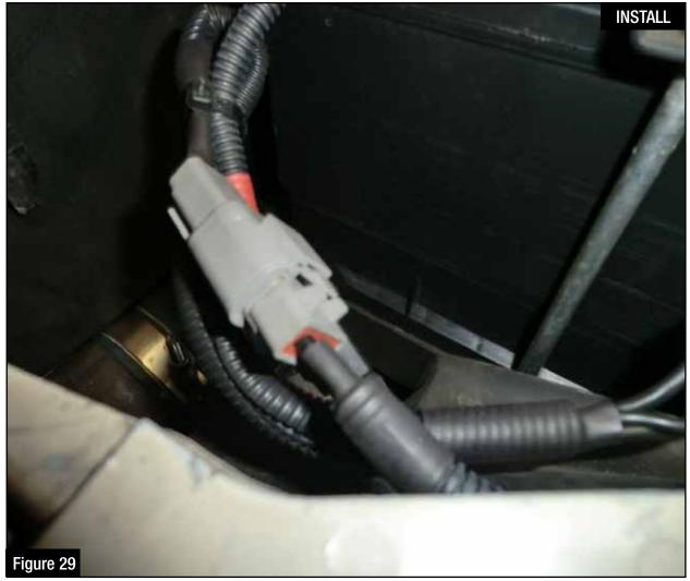
Step 33: Plug the supplied pressure switch harness into the Deutsch connector on the power harness.
