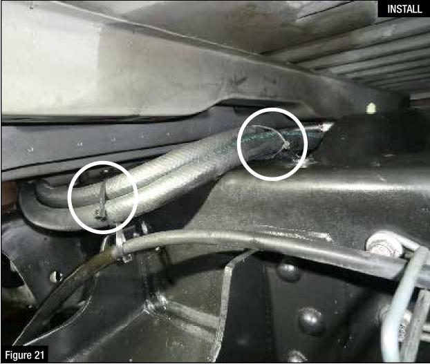
Step 22: Using the supplied nylon cable ties, secure the new hoses (as shown above).
