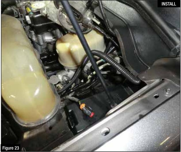
**Step 26:** Run the other end of the supplied wiring harness along the frame to the engine compartment. Secure using supplied nylon cable ties.
