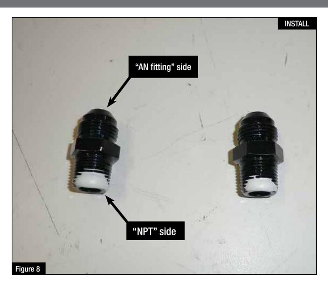
Step 10: Apply Teflon tape with PTFE or Teflon paste with PTFE to the 2 x 3/8" NPT to -8 AN fittings.
