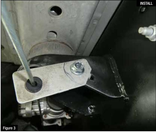
**Step 4:** Remove the bolt holding the emergency brake cable guide from the truck.
