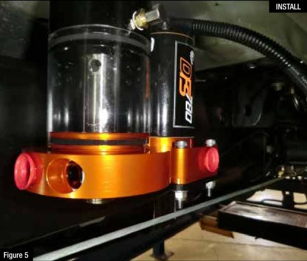
Step 6: Connect the manifold to the bracket using the four (4) supplied M6x1.0 x 50mm bolts,M6 washers, fiber washers and M6 flange nuts. The fiber washers go between the manifold and the bracket.
