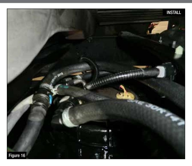
Note: This is what the top of the tank should look like after all the supplied hoses are connected.
