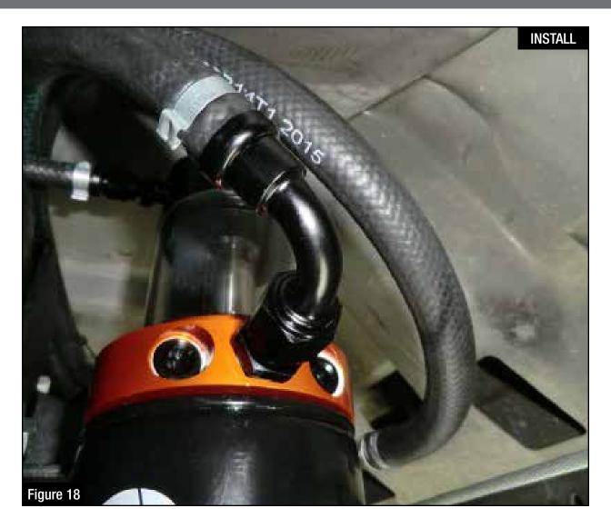
Step 19: Install the fuel outlet hose (90° black "AN" fitting) onto the fuel outlet port of the DFS780.
