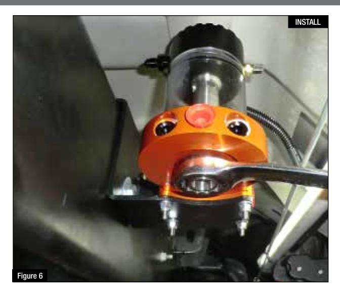
**Step 8:** Turn the sight glass to the desired angle and using a 1-1/4" wrench, tighten the center nut under the DFS780 manifold.
