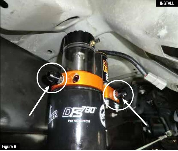
Step 11: Install the 2" x 3/8" NPT to -8 AN fittings into the DFS 780 (as shown above).
