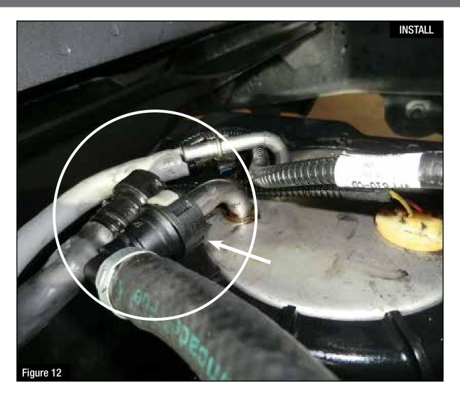
**Step 14:** Install the supplied fuel inlet hose (shown below with silver 90° "AN" fitting) onto the male side of the stock fuel tank connection.
