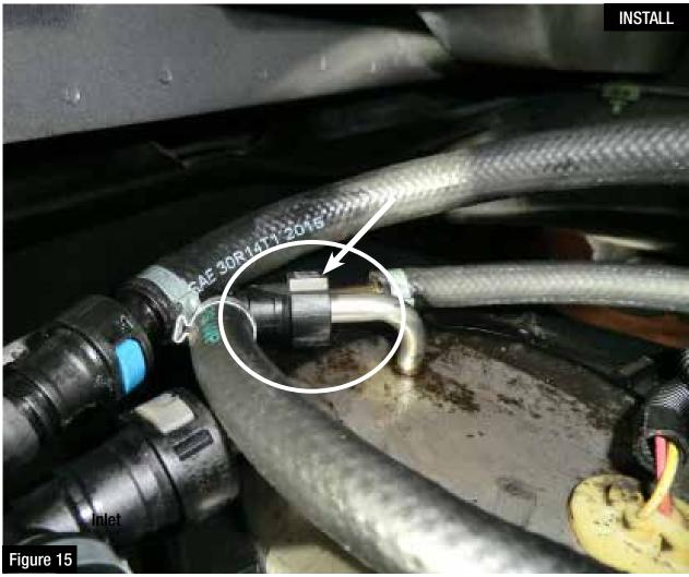
**Step 17:** Install the opposite side of the supplied return line to the male connection on the stock fuel tank connection (as shown below).
