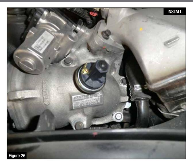
Step 29: Install the supplied pressure sensor onto the intake manifold (1/8" NPT).
