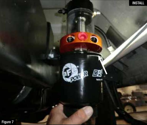
**Step 9:** Using a light oil, lube the gasket on the fuel filter and install on the manifold. Thread the supplied water separator bowl onto the supplied fuel filter.
