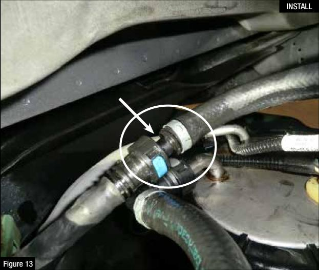
**Step 15:** Install the supplied fuel outlet hose (shown below with black 90° "AN" fitting) onto the female side of the stock feed line.
