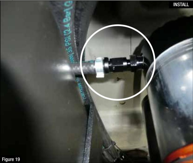
Step 20: Install the supplied fuel return hose (-4 AN fitting) onto the top of the DFS780.
