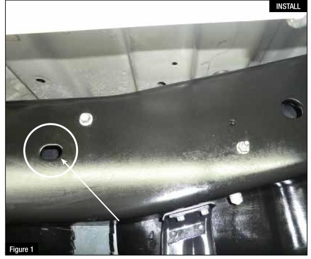
Step 1: You will need to loosen the bed or drop the fuel tank to begin installation of the DFS780 Fuel pump.
