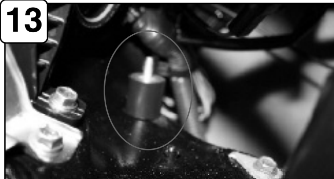
13 Install and tighten isolation mount to frame.
