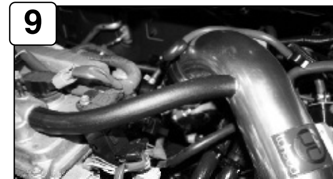
Remove engine cover using 10mm socket or wrench. Remove stock crank case line and replace with provided 5/8" hose. Re-install engine cover and tighten.
