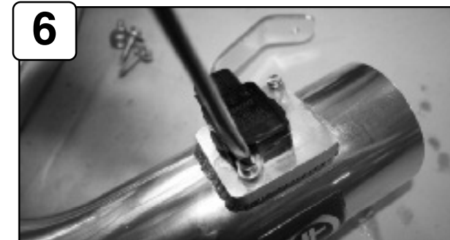
Install MAF sensor to upper intake tube assembly and secure using provided M4 screws.
