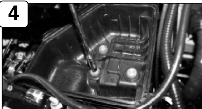
With 10mm socket or wrench loosen the 3 bolts holding in bottom half of air box and remove.
