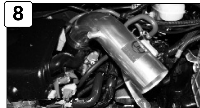
Install upper intake tube assembly into vehicle with provided reducer coupling and clamps. Do not tighten.
