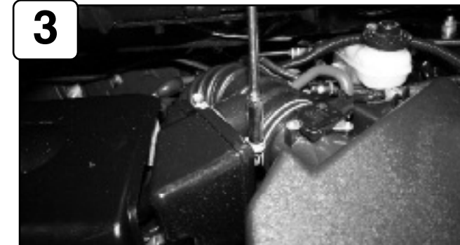
Disconnect MAF sensor and loosen clamp using 10mm socket or wrench. Unclip upper half of air box and remove. Loosen clamp with pliers on throttle body and remove stock intake tube.
