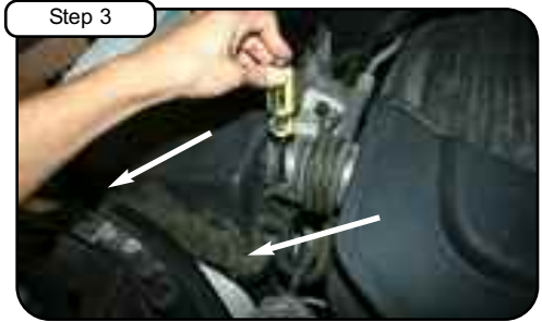
With 5/16" nut driver, loosen clamp at OE airbox. Detach the two factory clips holding the top of the OE airbox.
