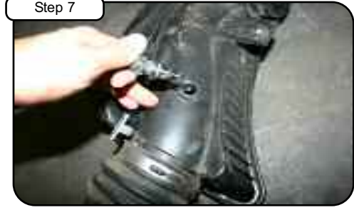
Remove the factory air temp sensor from bottom of the OE intake plenum box. Set aside to be re-installed on to new aFe intake tube.
