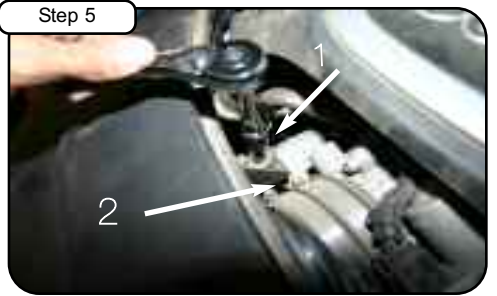
1) With 10 mm socket or wrench, loosen the 10mm bolt holding the factory intake plenum box. 2) With 5/16" nut driver loosen OE factory clamp at throttle body.
