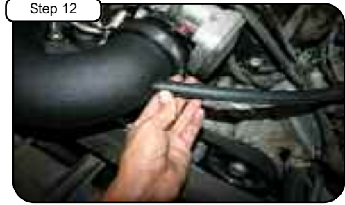
Carefully remove OE breather line. Replace with 1/2" hose supplied, insert one end onto tube and other onto breather fitting. Use the supplied mini clamps.
