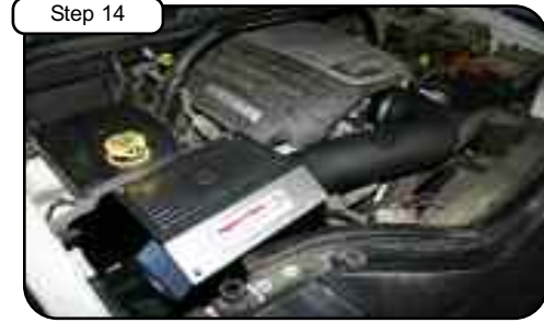
Place enclosed CARB EO sticker on a clean/smooth surface on or near the device. EO identification label is required in passing the Smog Check Inspection. The installation is now complete. Periodically Check all clamps and connections. Thank you for choosing aFe!
