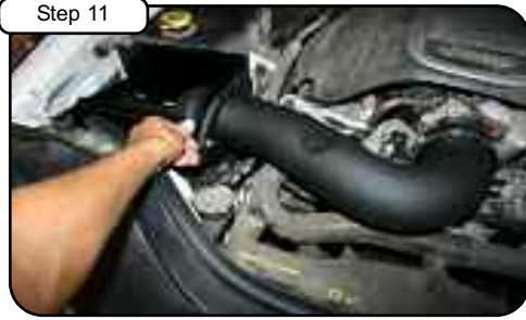
Gently place the new tube and housing into vehicle. At housing, re-attach the two OE clips from bottom half of airbox to the new aFe housing. Tighten clamp on coupler at the tube side.
