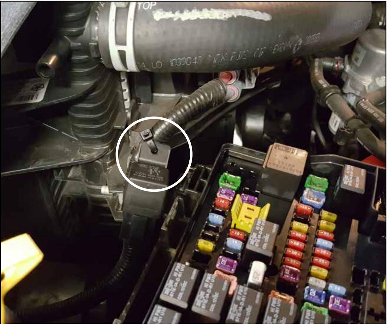
Step 32: Secure the supplied relay using a supplied nylon cable tie.
