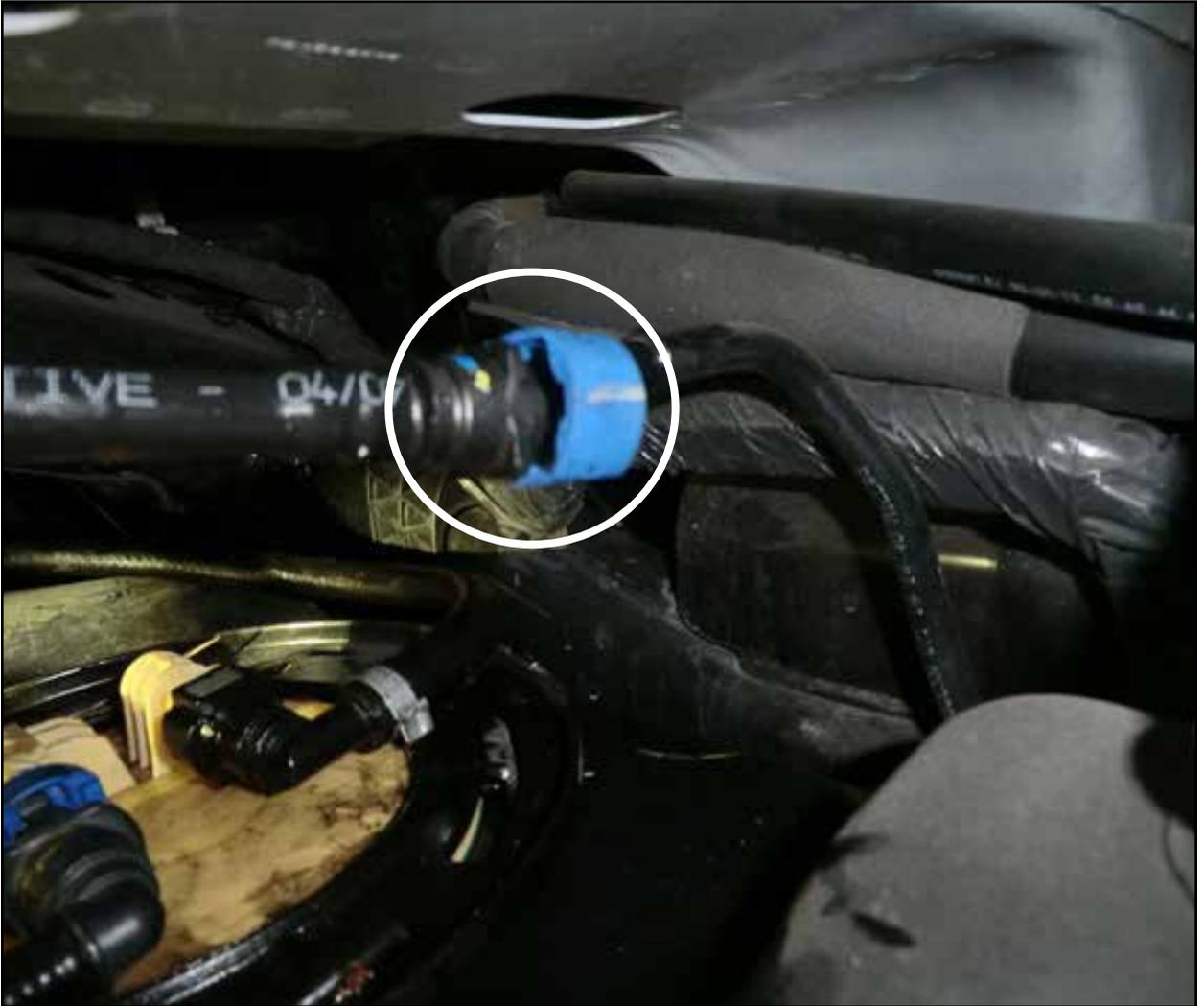
Step 11: Disconnect the factory fuel line from the fuel line near the frame (blue).
