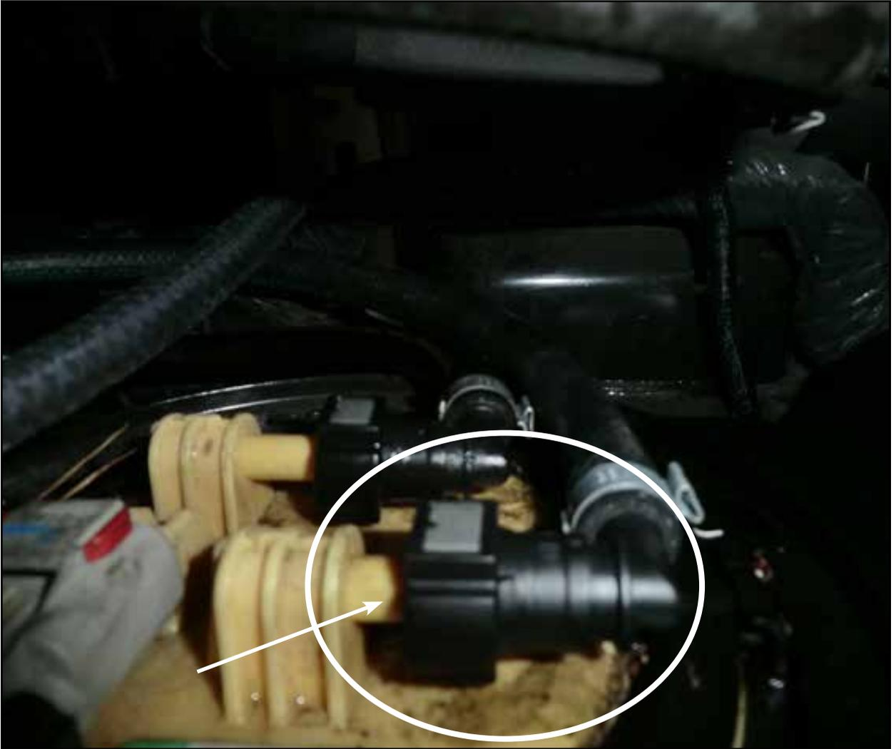
Step 16: Install the 90° female quick disconnect fitting onto the male fuel return connection on the tank.
