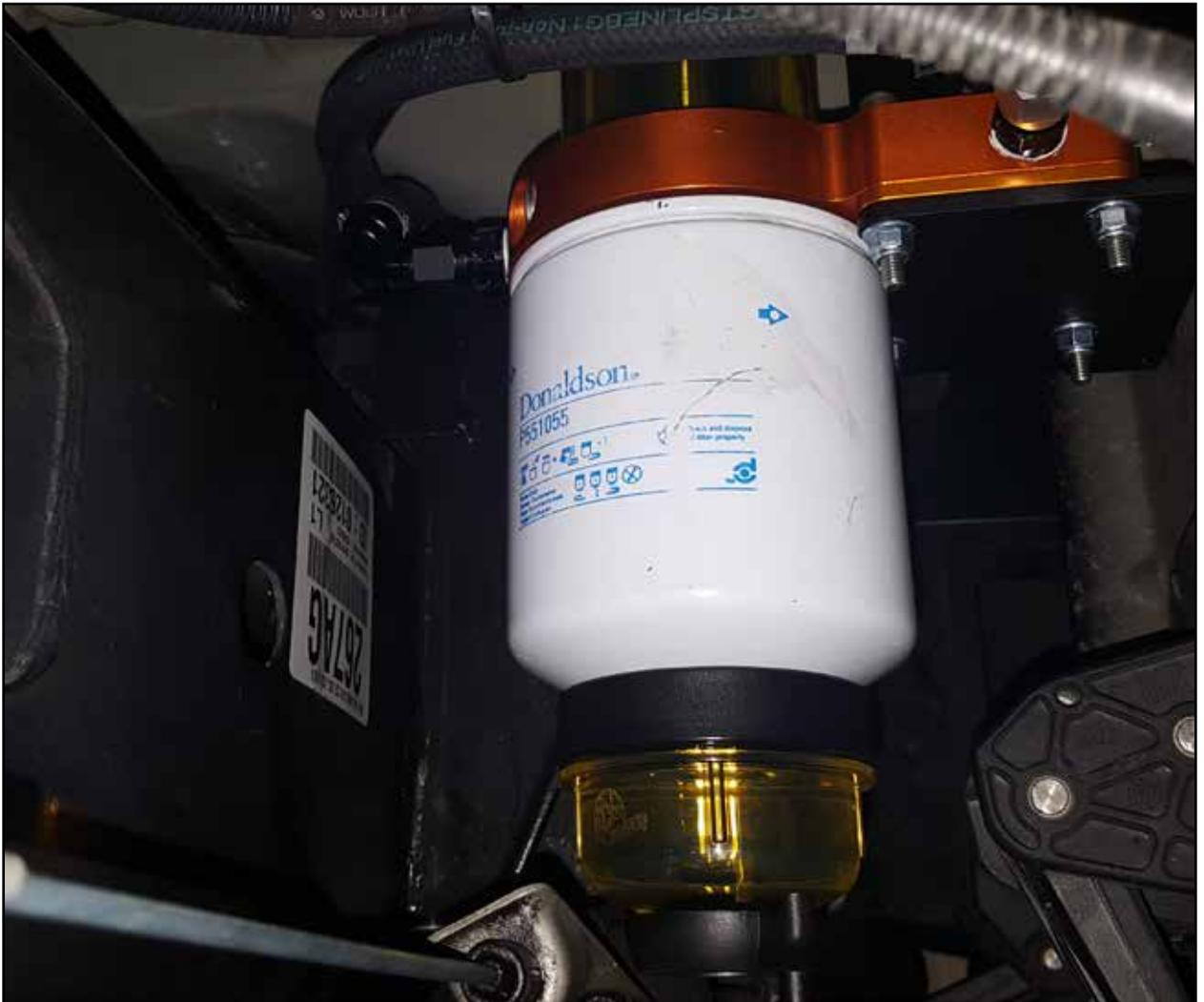
Step 40: Turn the key to the “Run” position and watch to see if the sight glass fills with fuel. If the sight glass does not fill with fuel, use the tank valve (on the top of the sight glass cover) to release any trapped air. If the sight glass still does not fill, try starting the engine.
