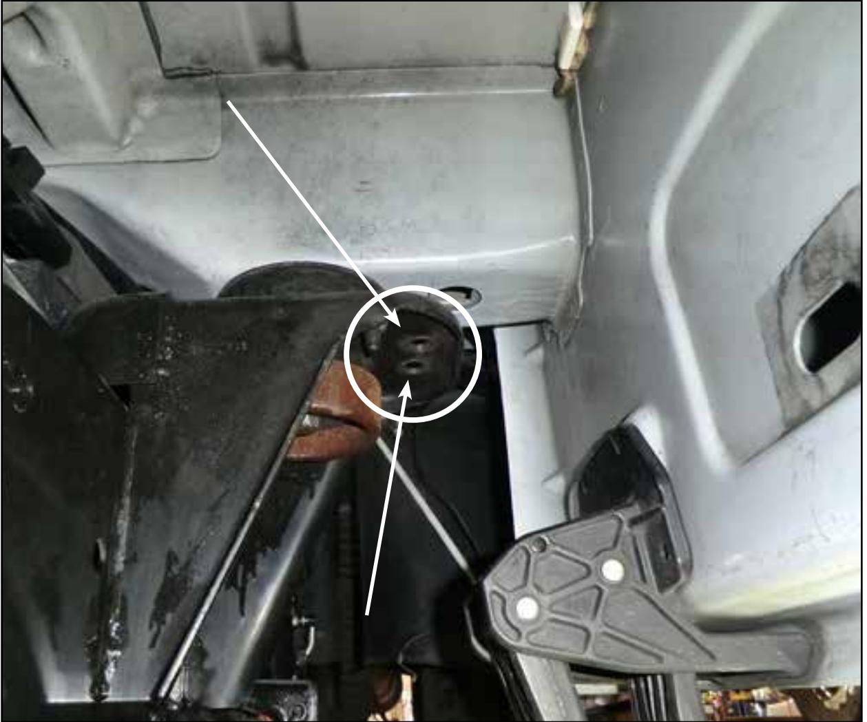
Step 1: Looking at the driver's side of the truck, at the back of the cab on the outside of the frame rail, you will see a body mount with two (2) holes on the outer lip.
