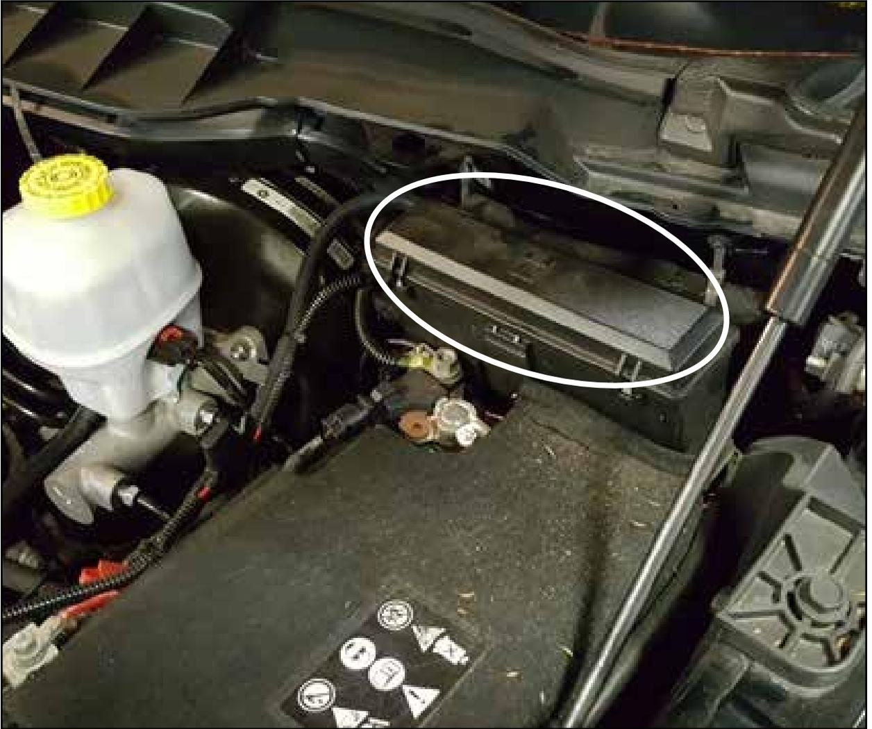
Step 28: Reinstall the power distribution box back in its factory location.
