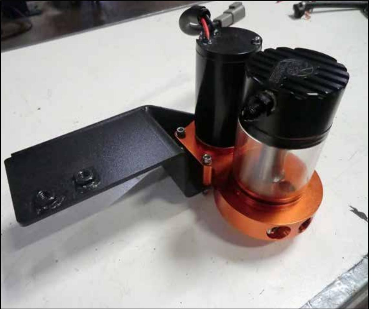
Step 3: Mount the supplied fuel manifold assembly to the carbon steel frame bracket using the supplied hardware and tighten.
