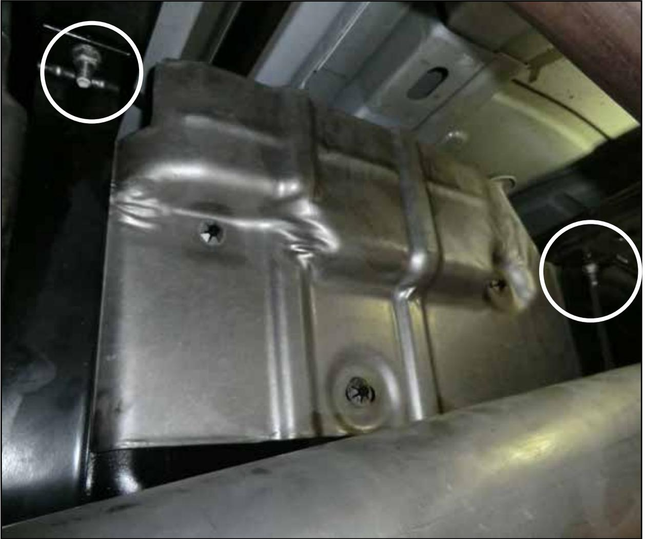
Step 9: It will be necessary to lower the fuel tank or remove the bed to gain access to the top of the fuel tank.
