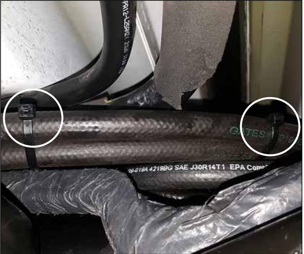
Step 21: Using the supplied nylon cable ties, secure the new hoses (as shown above).
