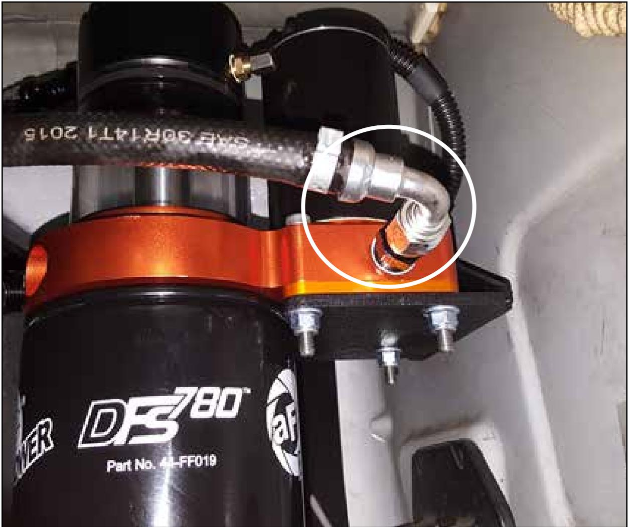
Step 18: Install the fuel inlet hose (silver 90° -6 AN fitting) onto the male -6 AN fitting on the fuel inlet port of the fuel manifold assembly and tighten.
