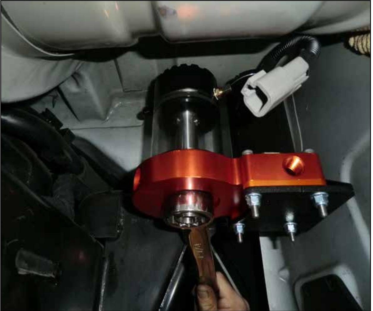
Step 5: Turn the sight glass to the desired angle and using a 1-1/4" wrench, tighten the center nut under the fuel manifold assembly.
