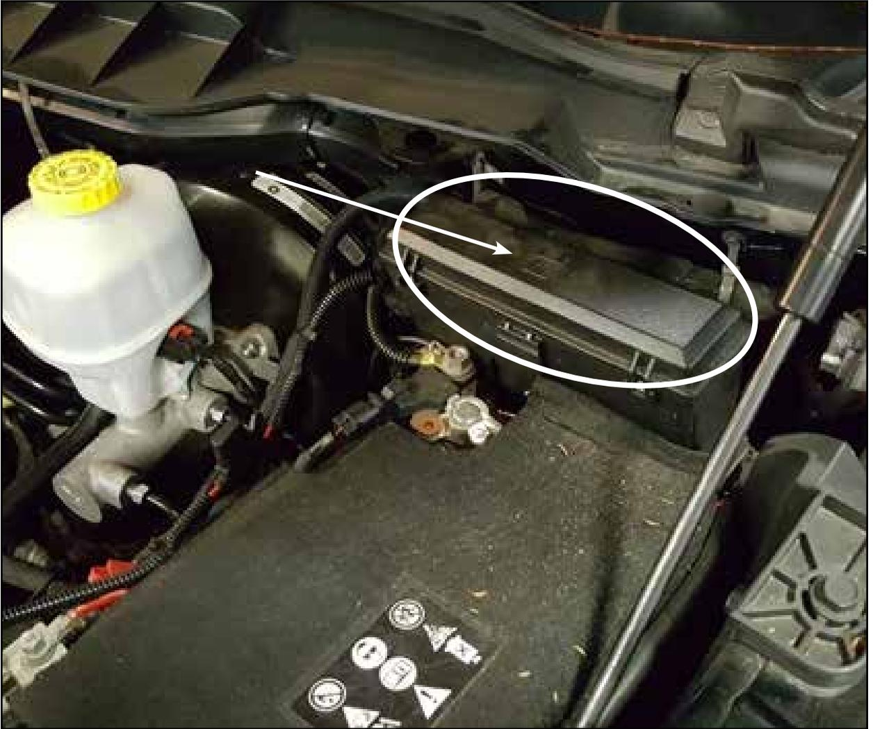
Step 26: Move the power distribution box out of the way by carefully pulling straight up on it.
