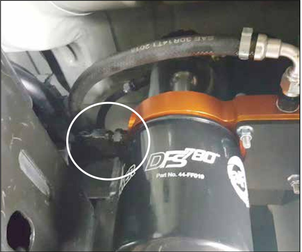
Step 19: Install the fuel outlet hose (black 90° -6 AN fitting) onto the male -6 AN fitting on the fuel outlet port of the fuel manifold assembly and tighten.
