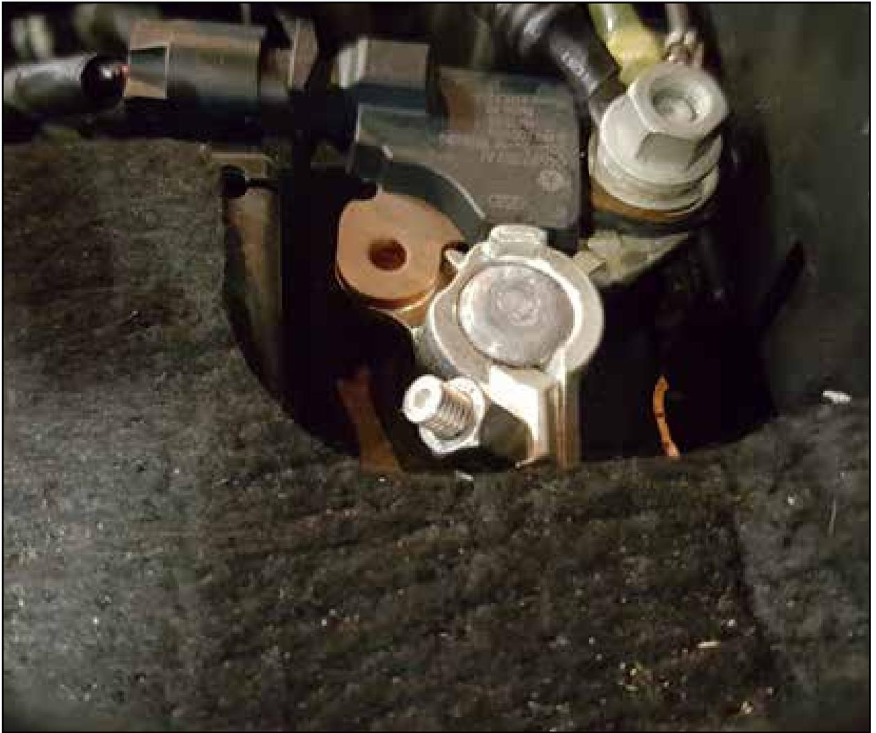
Step 30: Connect the black wire ring terminal on the power harness to the negative side of the battery.
