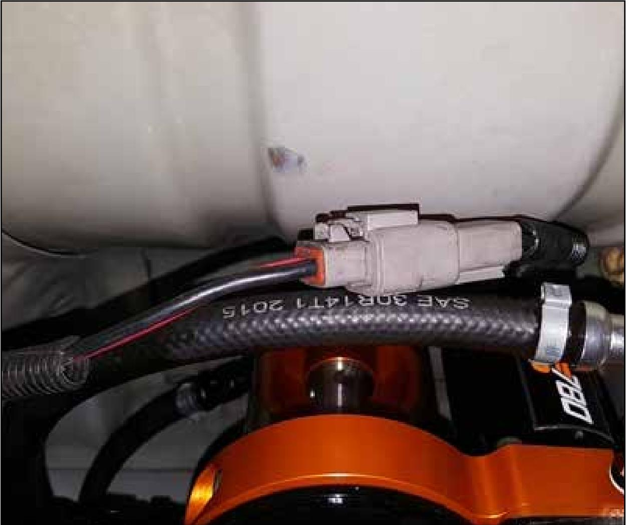
Step 22: Plug the Deutsch connector on the supplied power harness into the mating connector on the fuel pump motor.
