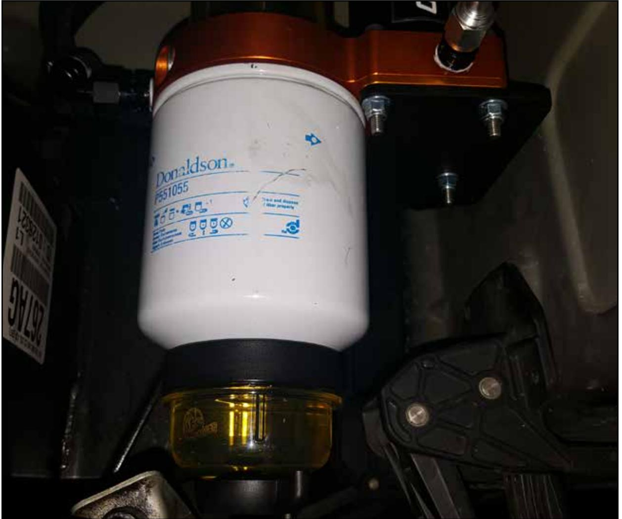
Step 6: Using a light oil, lube the gasket on the supplied fuel filter and install on the fuel manifold assembly. Thread the supplied water separator bowl onto the fuel filter.
