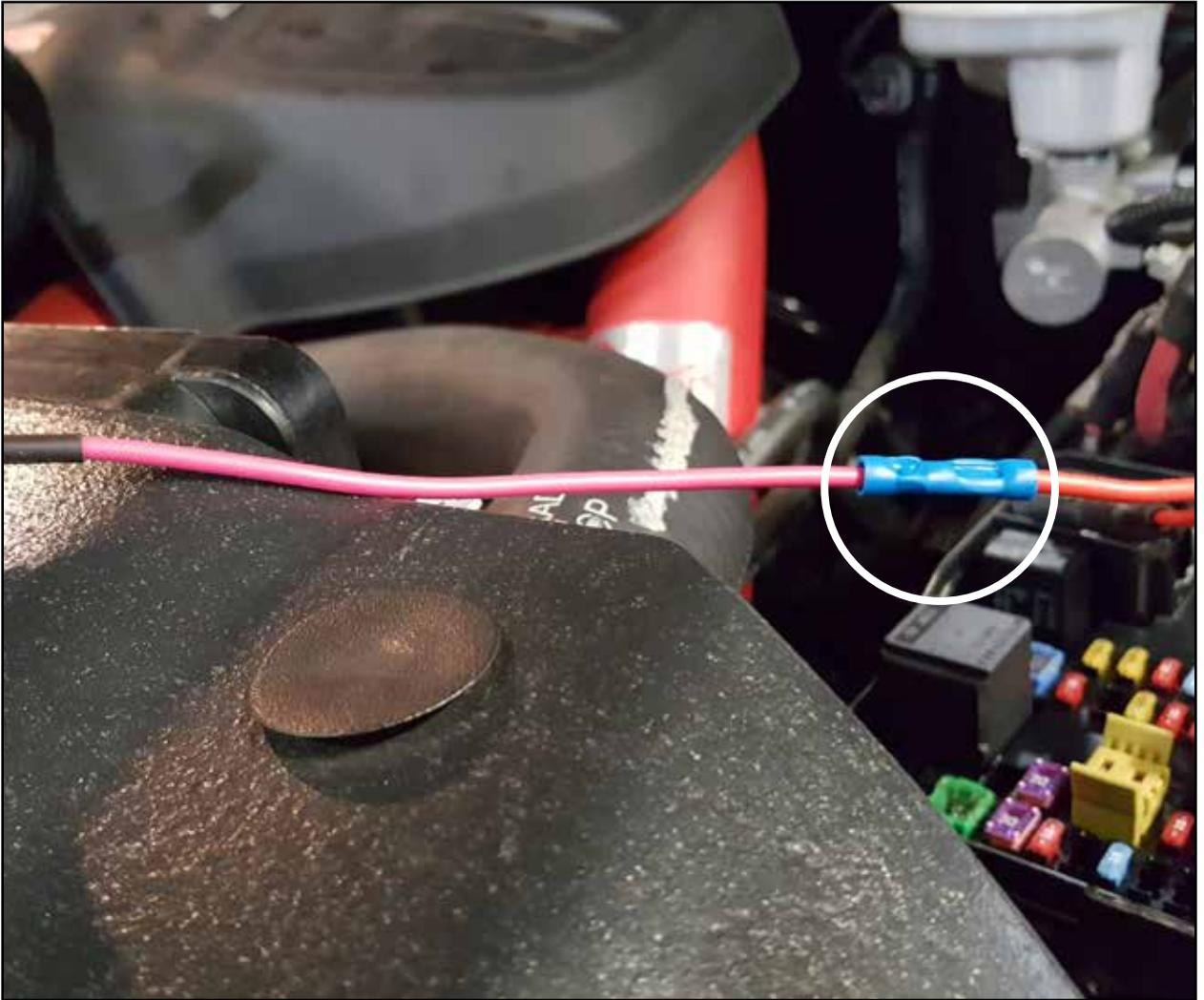
Step 35: Attach the power wire from the relay to the add a harness fuse adapter.
