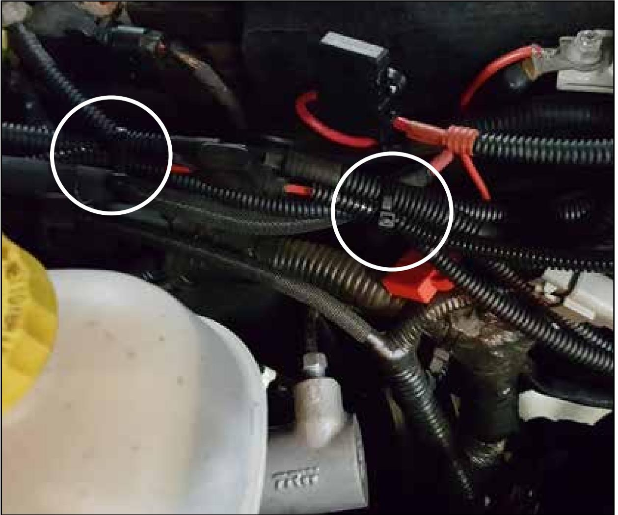
Step 38: Carefully route the power wire outside the fuse box and reinstall the cover (making sure not to pinch the wire).
