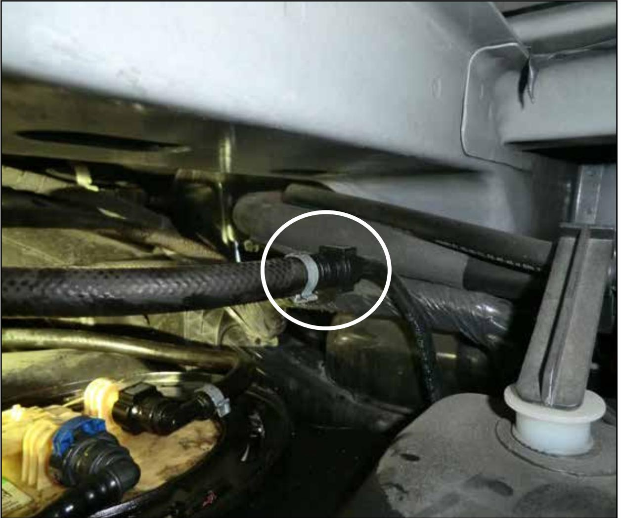
Step 14: Install the female quick disconnect fitting on the supplied fuel outlet hose (black 90° -6 AN fitting - shown below) onto the male side of the stock fuel feed line.
