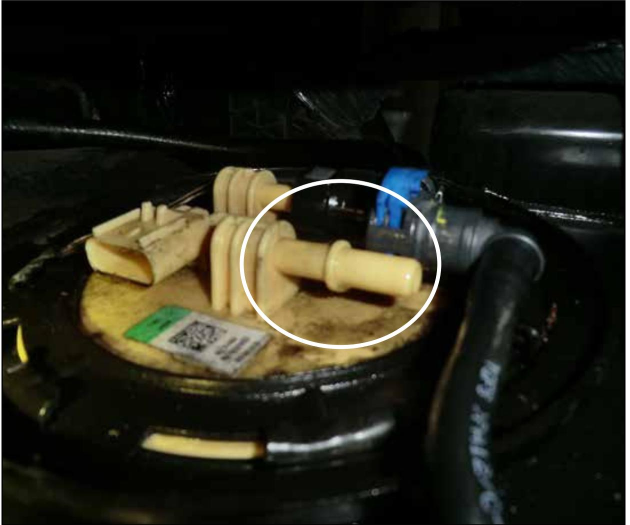
Step 15: Disconnect the factory return fuel line from the return connection on the tank.
