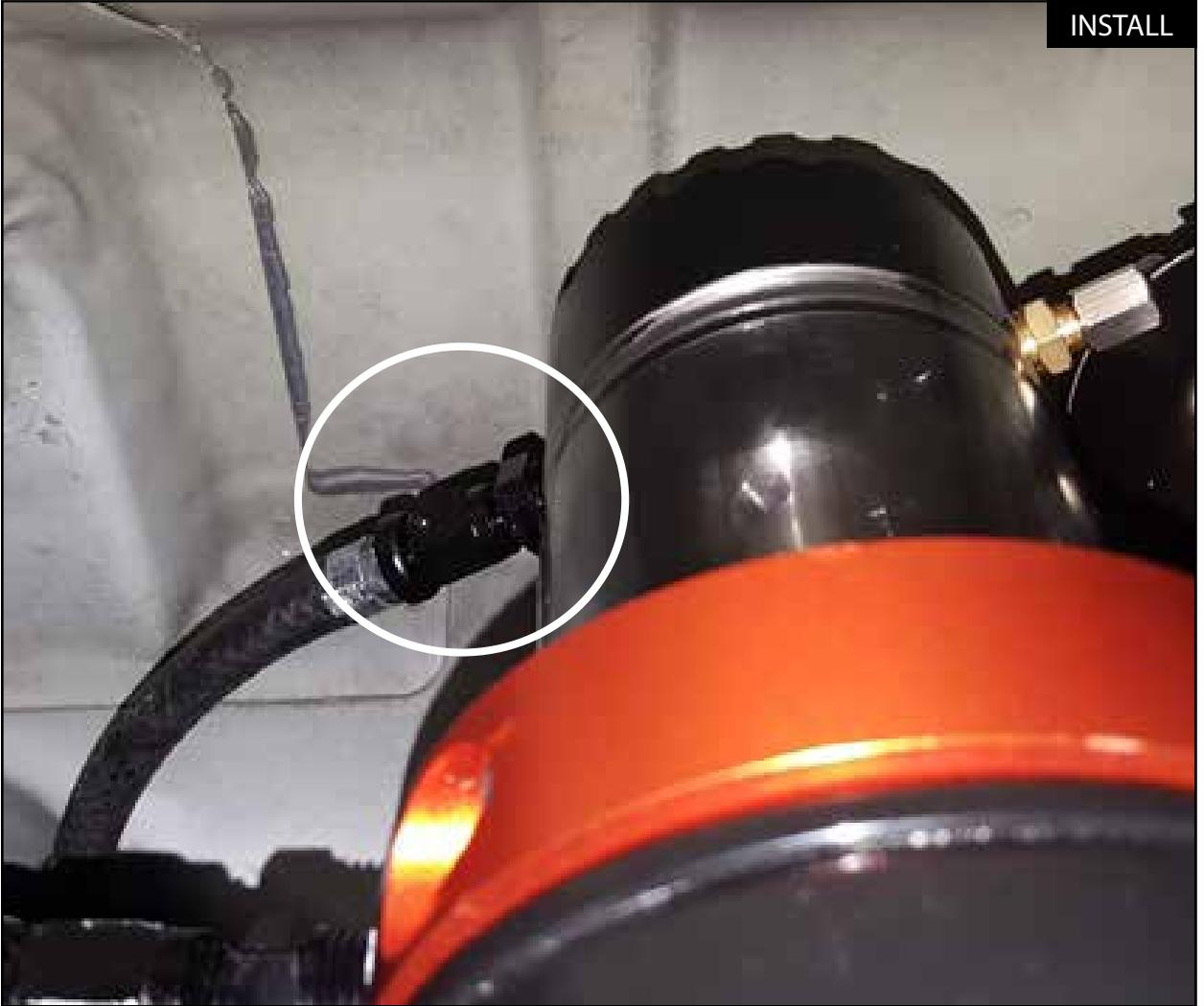
Step 20: Install the fuel return hose (-4 AN fitting) onto male -4 AN fitting on the top of the sight glass cover and tighten.
