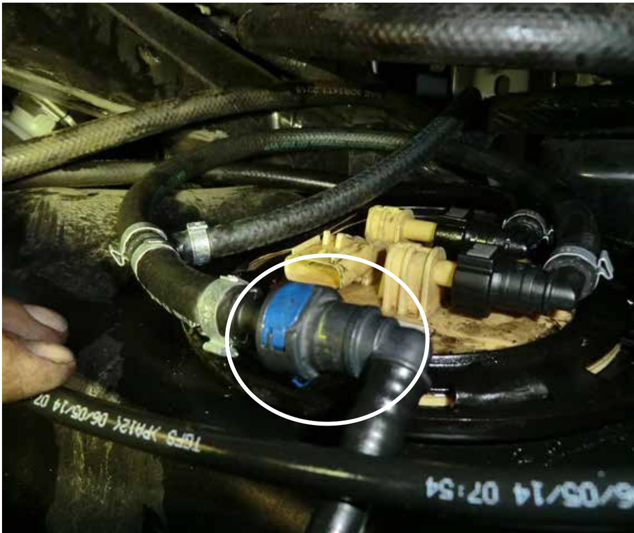
Step 17: Install the straight male quick disconnect fitting on the supplied fuel return hose into the female side of the stock fuel return line.
