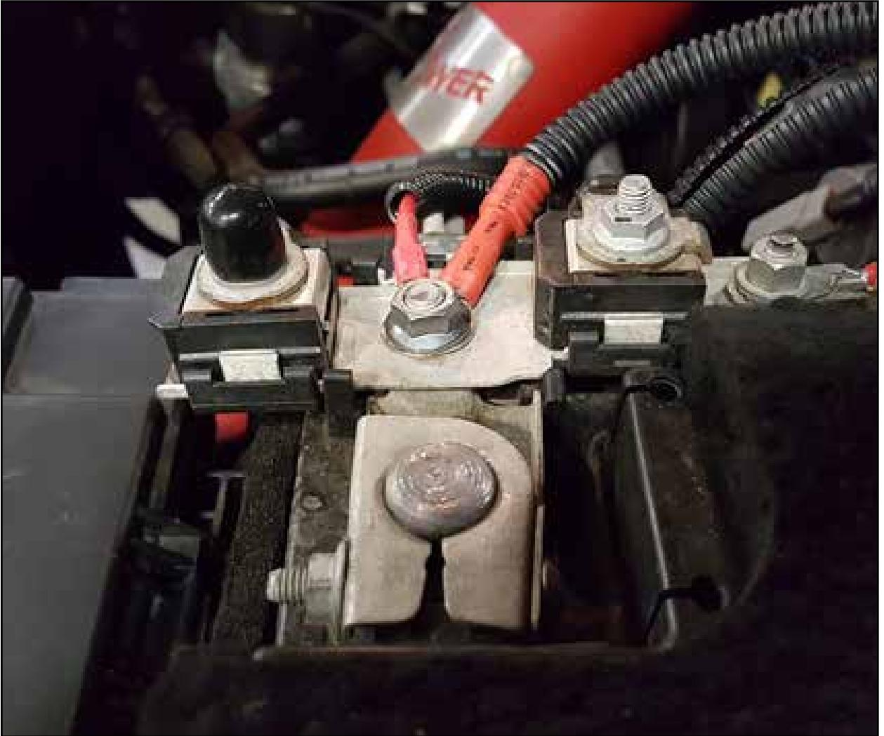
Step 29: Connect the red wire ring terminal on the power harness to the positive side of the battery.
