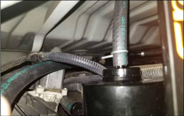
Step 15: Carefully route the ¼" hose to the DFS780 Pro fuel pump, making sure not to kink the hose or allow it near moving parts. Carefully mark and then cut the hose to the correct length. Using the supplied 7/16" spring clamp, attach the hose to the nipple on the top of the air chamber on the DFS 780 Pro fuel pump assembly.
