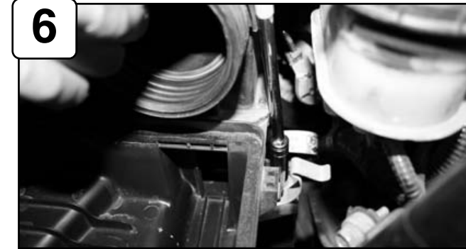
Using a 10mm socket or wrench, remove the mounting bolt on the back of the lower intake box.
