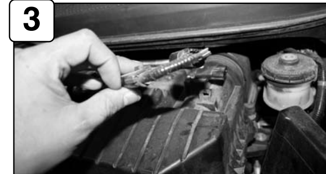
Unplug the MAF sensor harness.
