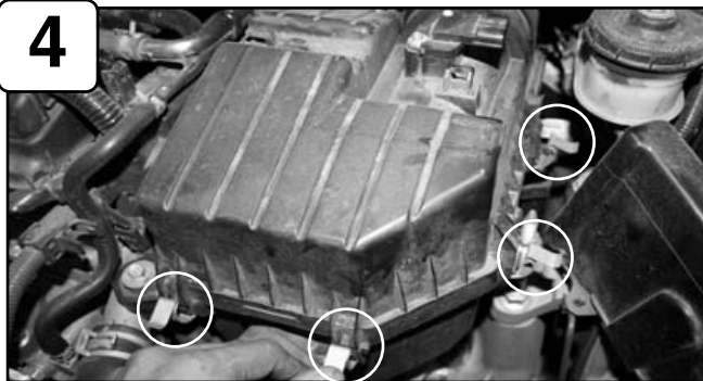
Disconnect all retainer clips and remove the upper intake box.
