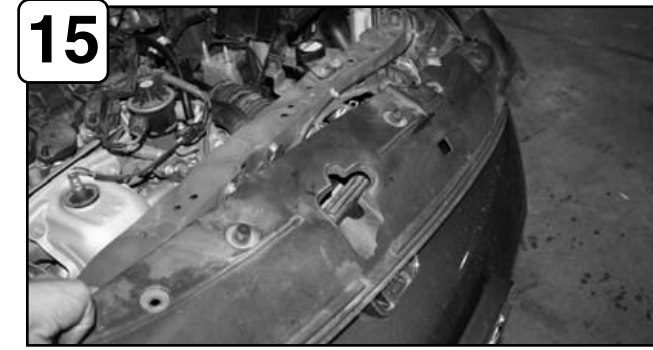
15 Remove the front bumper. Start with removing all the push clips holding the upper splash guard onto the vehicle. When all are removed, gently pull the splash guard off of the hood latch and put it aside.
