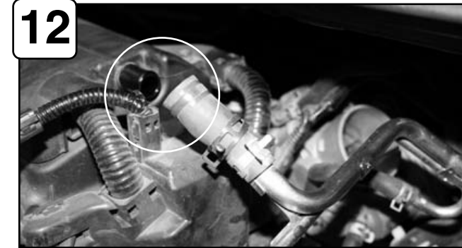
12 With pliers, remove the pressure clamp holding the crank case breather line to the valve cover and pull it off.
