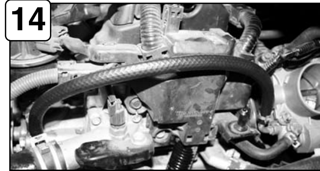
14 Replace the existing oem hose line with the new hose line re-using your existing clamps.
