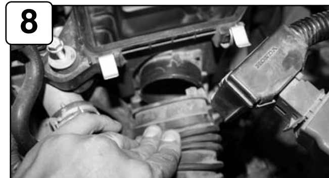
Pull the ram air duct tube off of the lower intake box.
