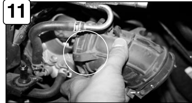
11 Disconnect the clamp holding the intake tube to the throttle body and pull the wire loom off of the tube and put aside.
