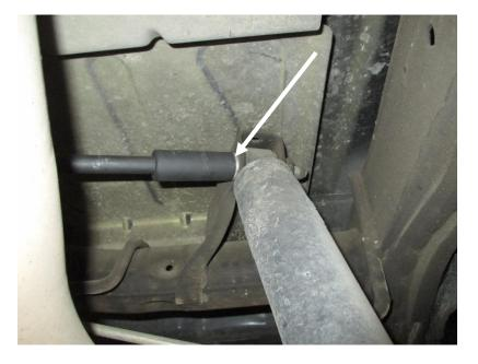
6. Using the stock nuts and bolts, install your new shocks with the bottom eyelet first and the upper eyelet second.
