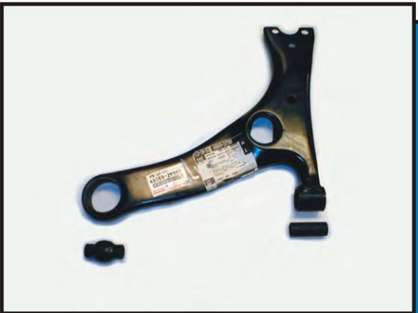
Note: Make sure to thoroughly grease the tapered face of the #3374 bushing to aid in installation.
