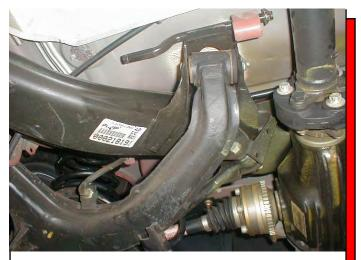
The inner position bushing has an outer plastic shell that needs to be pressed out. The I.D. of control arm is Ø1.608, use something smaller when pressing out the old bushing. Trim off the plastic flange of the shell and press out the bushing. Apply grease to all metal parts that contact the polyurethane bushings. Grease P/N's 2598 and sleeve P/N 15.10.180.39 and insert into the control arm.
