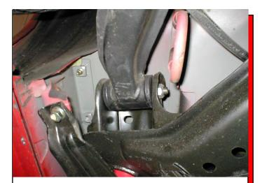
The outer position bushing has no outer metal shell that needs to be pressed out. The I.D. of control arm is Ø1.608, use something smaller when pressing out the old bushing. The O.E. rubber bushing is not bonded to the control arm. Trim off the flanges of the rubber bushing (both sides) and press out the bushing. Apply grease to all metal parts that contact the polyurethane bushings. Grease P/N's 2595 and sleeve P/N 15.10.180.39 and insert into the control arm.
